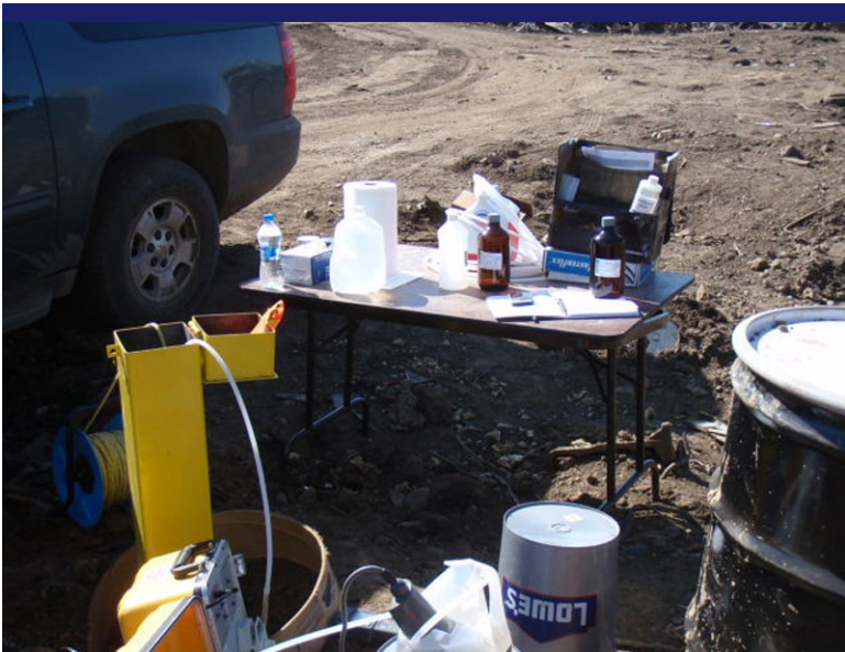
Photo 11 Low flow water sampling set up MW-2.
