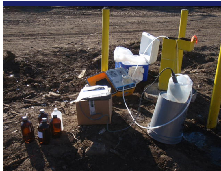
Photo 14 Set-up for MW-2 sampling.
