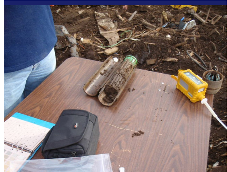
Photo 2 PID meter and first sample core from MW-4.
