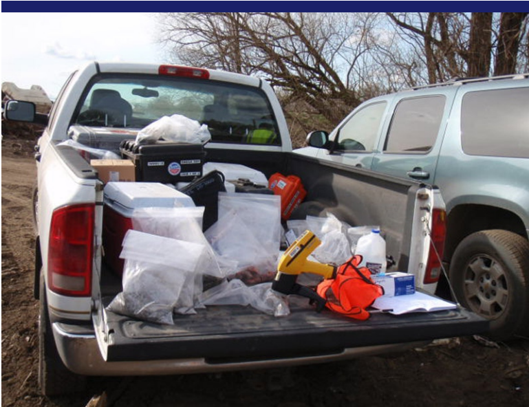
Photo 9 XRF gun and SB samples.
