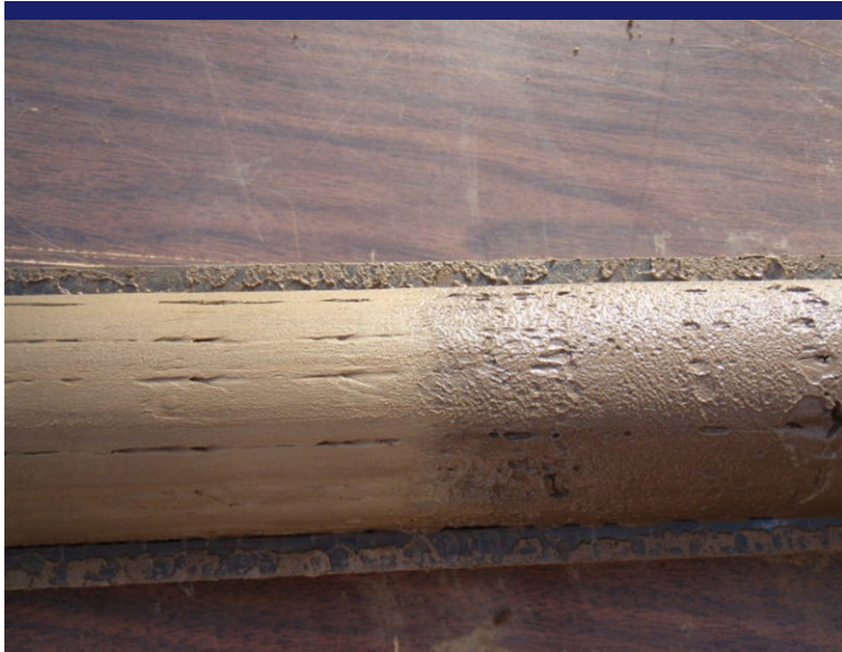
Photo 5 Drill core at 10 feet, water table barrier.
