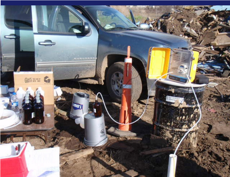
Photo 10 Sampling MW-4, duplicate and MS/MSD.
