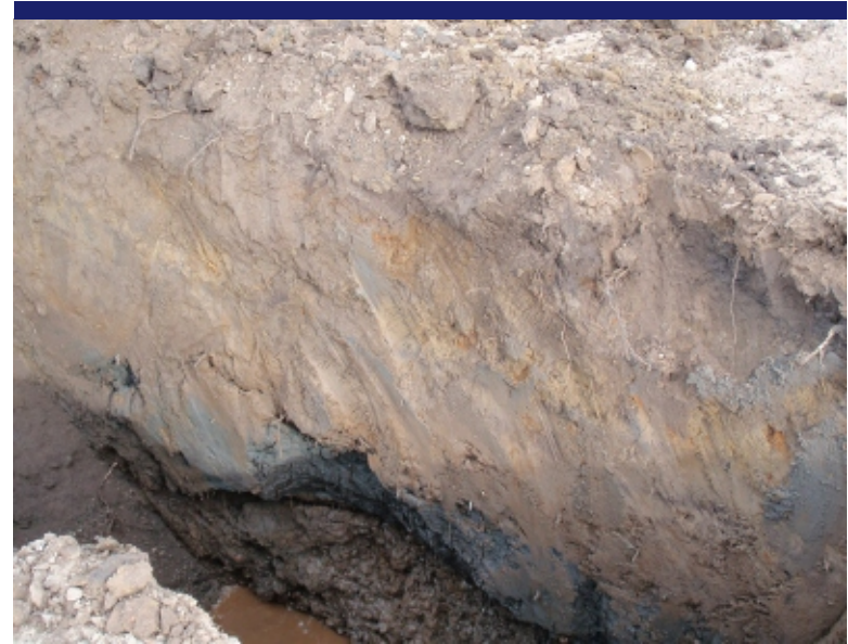
Photo 14 Sidewall of Test Pit 4. Soil horizons appear undisturbed.
