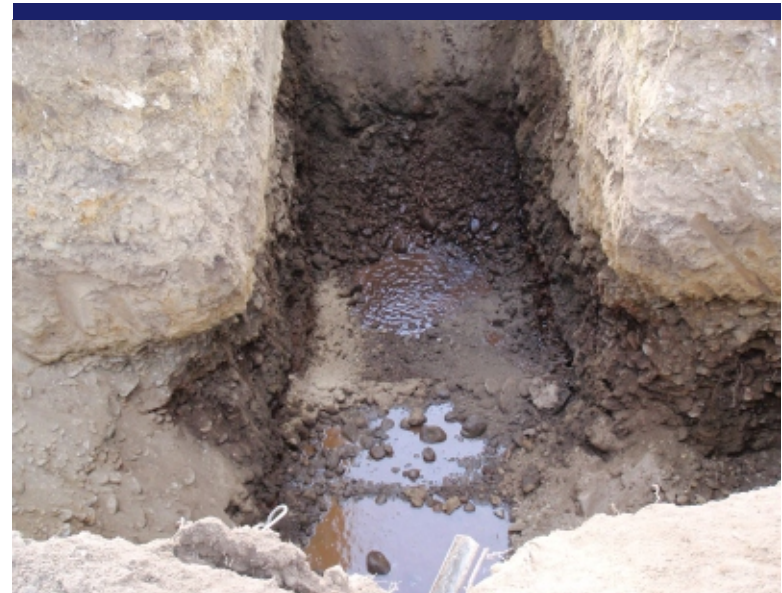
Photo 8 Striking groundwater in Test Pit 2. Note: No sheen visible.
