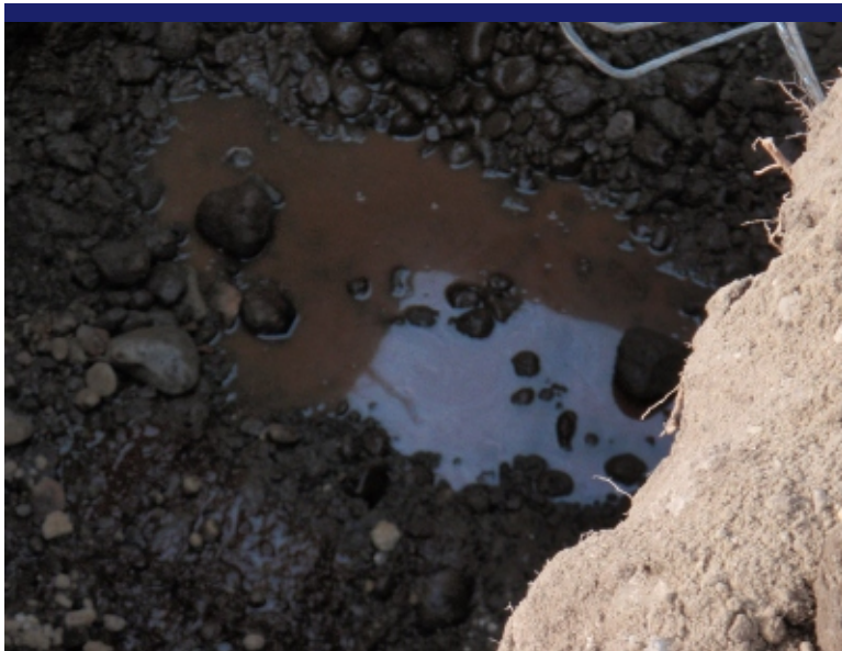
Photo 7 Sheen visible on groundwater in Test Pit 1.
