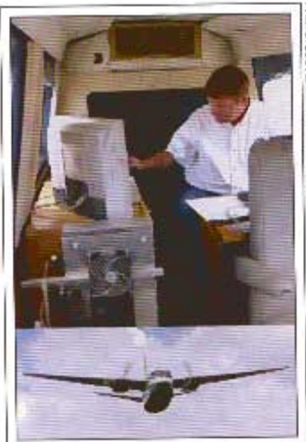
A technician measures readings from ASPECT infrared sensors mounted on an AeroCommander 680.
