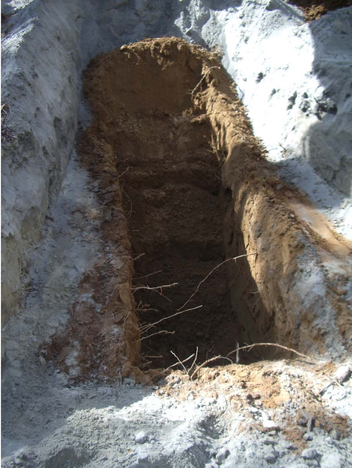
Photograph 4: Photograph of Test Pit TP-07. Note color difference between soil and tailings.
