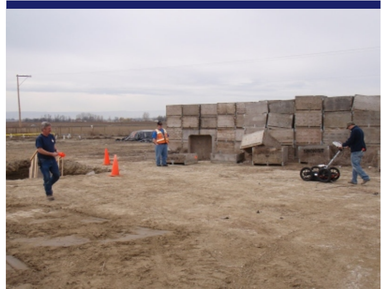
Photo 6 Ground penetrating radar identifying subsurface anomalies.
