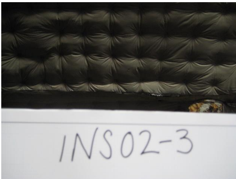
Ins-02-3_4 inch Duct Insulation
