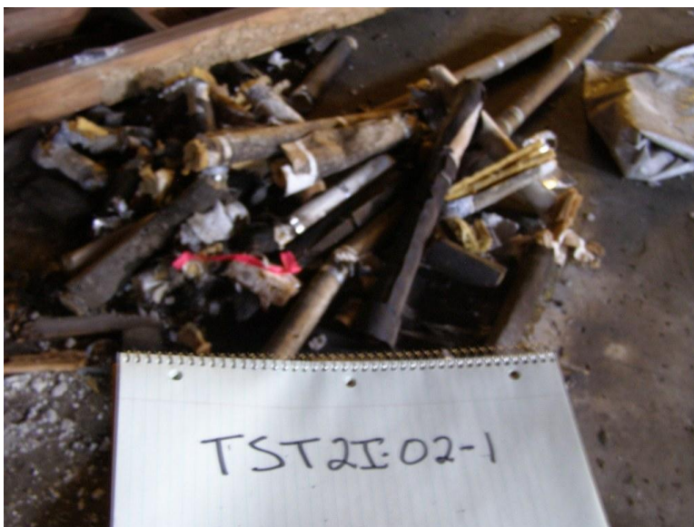
Tsi2i-02-1_2 inch White Wrapped Piping
