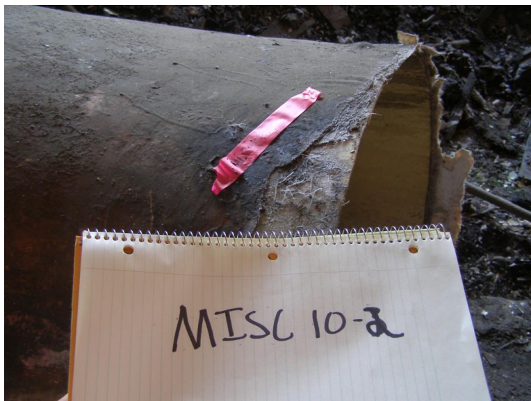
Misc-10-2_Fiber Wrapped Piping
