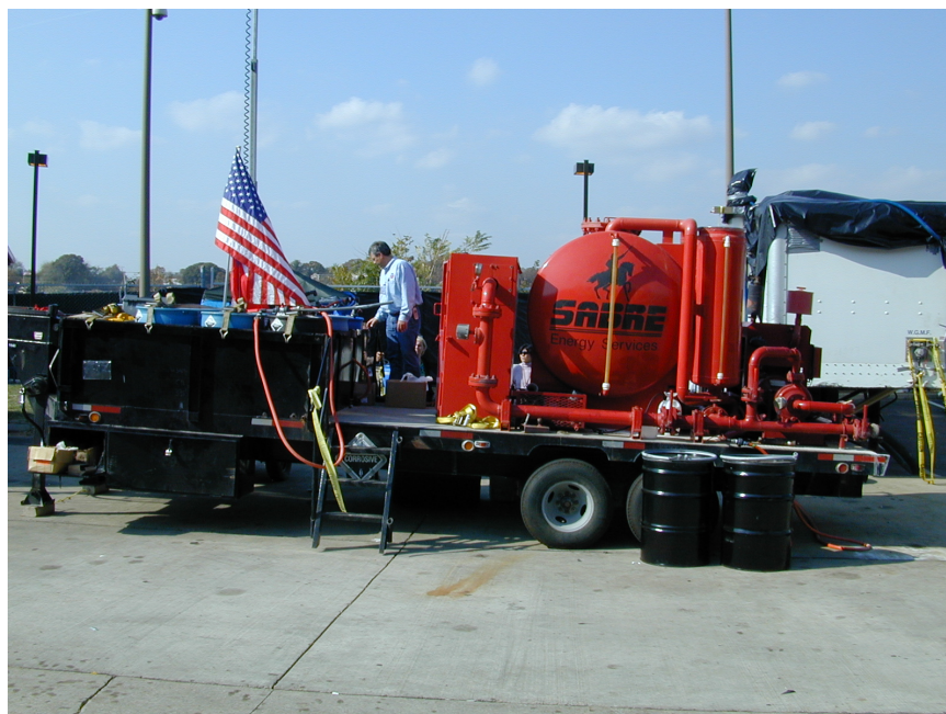
Figure 1. Chlorine Dioxide Generation System. The chlorine dioxide generation system used by Sabre Oxidation Technologies, Inc. for the onsite generation of the gas.
