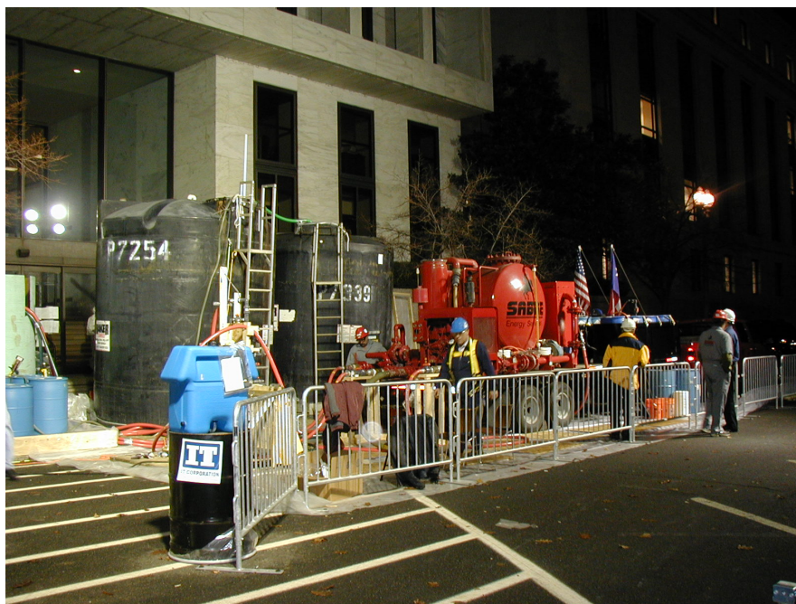
Figure 7. Chlorine Dioxide Generation System for HSOB. The onsite chlorine dioxide generation system for all HSOB operations.
