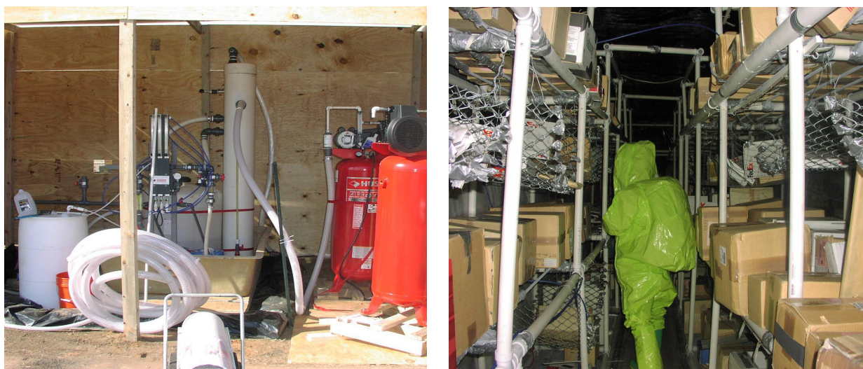
Figure 11. Chlorine Dioxide Generation System and Interior Operations. These two photos illustrate the chlorine dioxide generation system and the interior setup at the Beltsville remediation facility.
