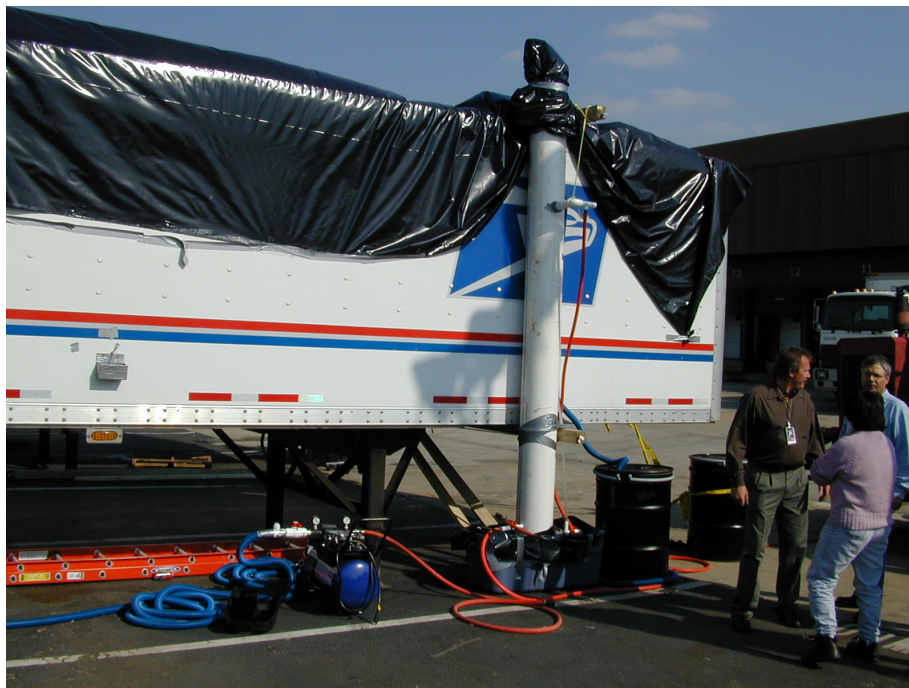
Figure 2. Chlorine Dioxide Remediation Test Trailer at the Brentwood P&DC. The cylinder in front is designed to eliminate excess chlorine dioxide and prevent its release into the atmosphere.
