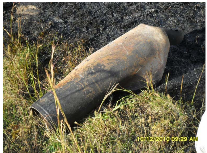
Figure 4 Exploded acetylene cylinder.
