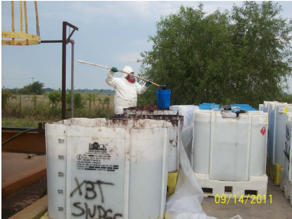
Sample collection of sludge for waste profiling (Photo# 103_3353).
