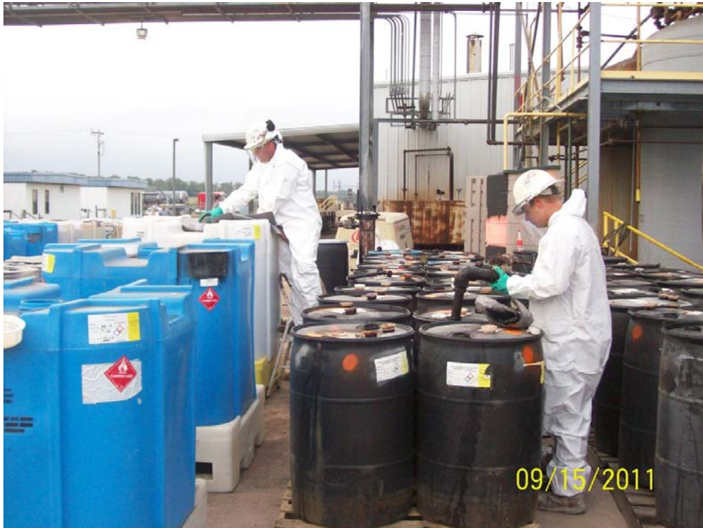
Filtration of DBFB/dibromotoluene mix, using a 50-micron filter (Photo# 103_3360).
