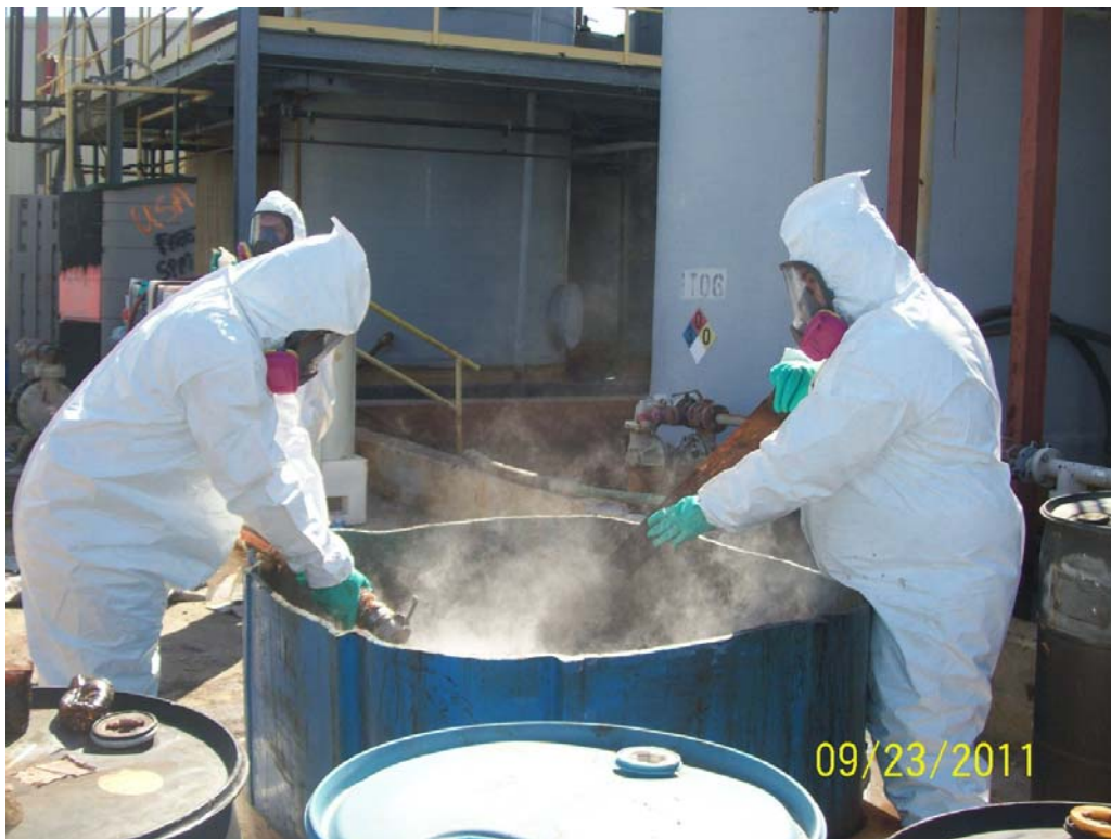
Neutralizing corrosive (low) pH liquids (Photo# 103_3423).
