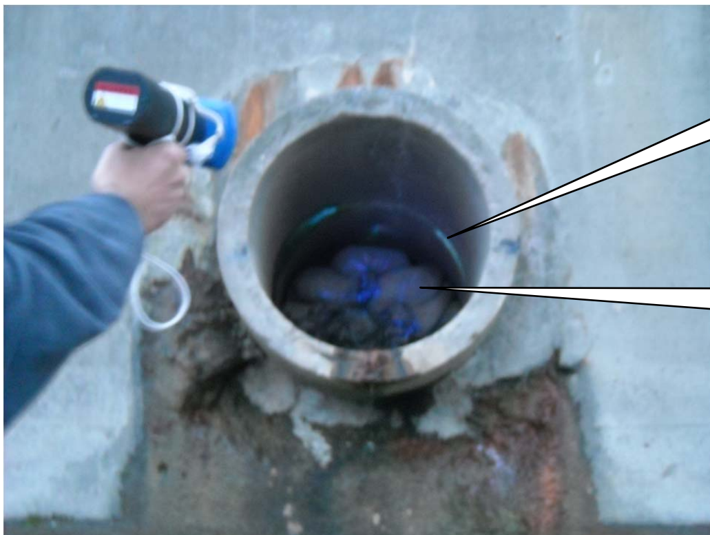
Light blue fluorescence within joint of piping
