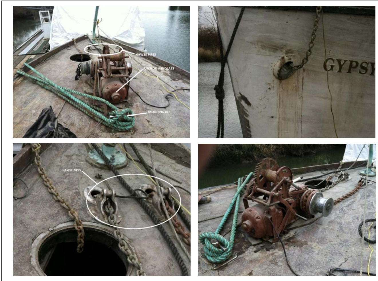
Gypsy Queen - anchor windlass, hawse pipe and bit arrangement
