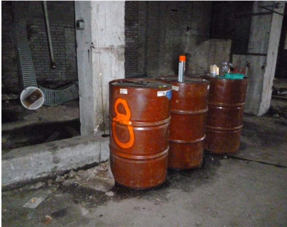
Photograph No.: 11 Photographer: Naren Babu Orientation: East TDD Number: TO-01-11-11-0027 Contract: EP-S5-10-10, OTIE Date: November 16, 2011 Site Name & Location: Rock-Tenn Site, Allegan County, Michigan. Subject: Drums with crude motor oil.
