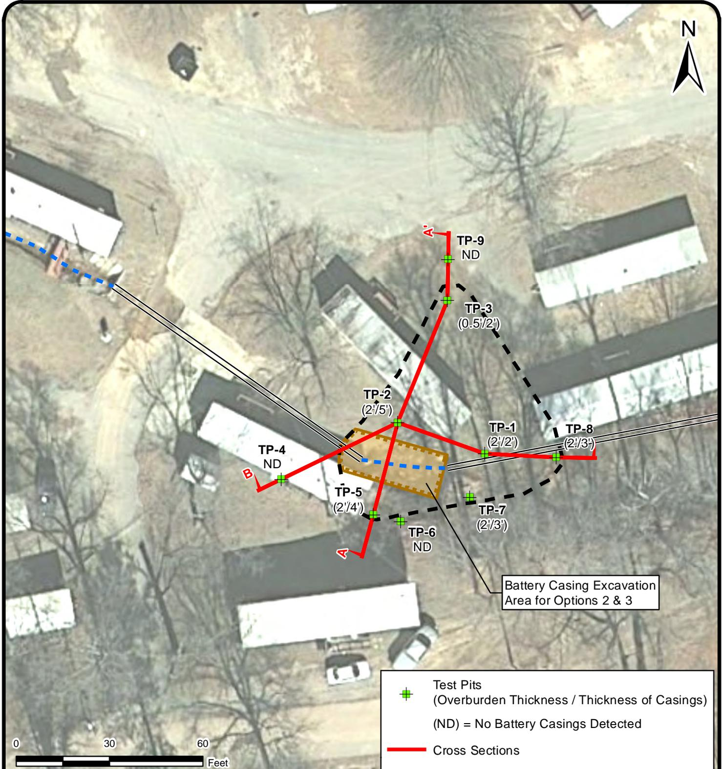
Battery Casing Excavation Area for Options 2 & 3
