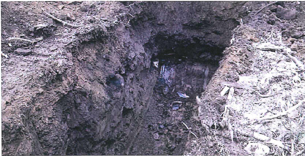
Subsurface contaminated material (coal tar) in a test pit at the Ironwood MGP Site (April 2012)
