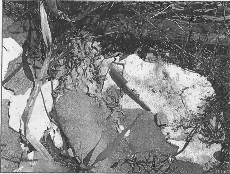
East-West Surveyors Line Sample No. DB-01 – Non-friable ACM TSI Mastic Debris
