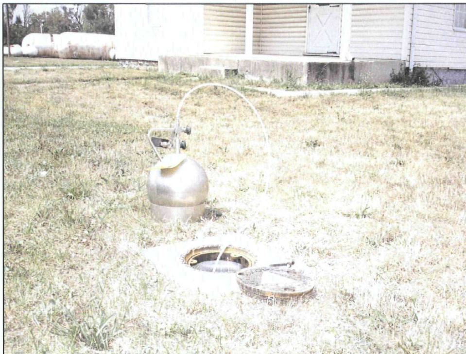
Photo 2: Soil Gas Sampling adjacent to residence on East River Road
