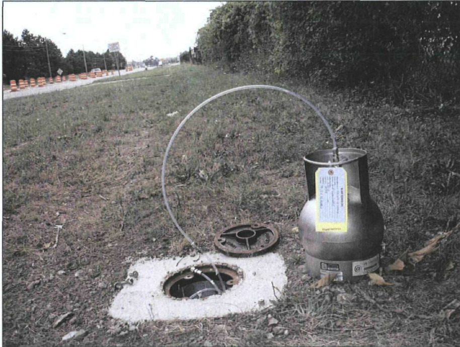
Photo 3: Soil Gas Sampling on Dryden Road
