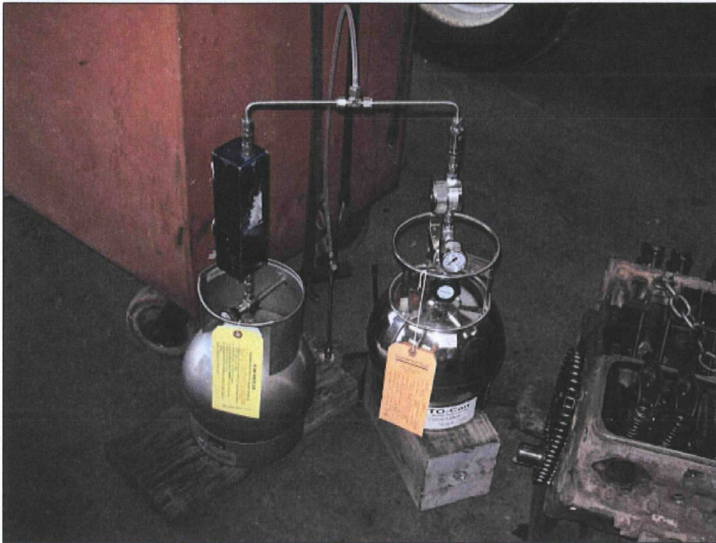
Photo 5: Sub-Slab Sampling at a Non-Residential building on Dryden Road
