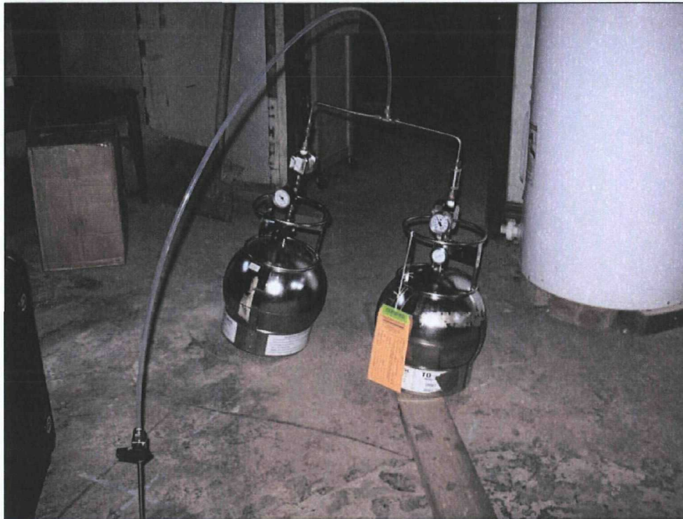
Photo 1: Residential Sub-Slab Sampling on East River Road
