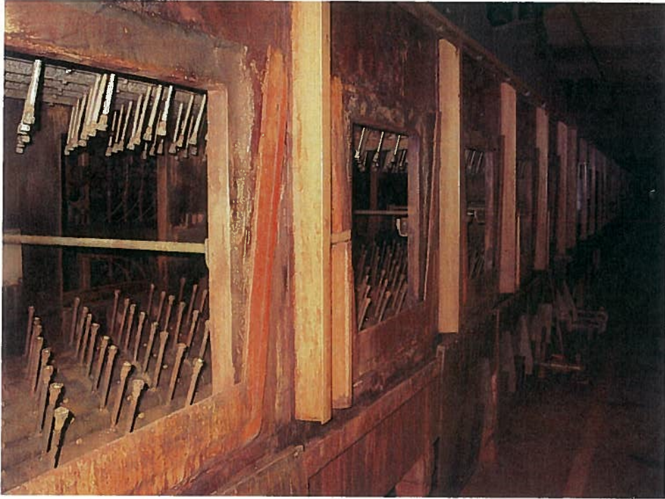
Photograph 17: The pH of the condensation located on this process line in room 5-128 is 1.
