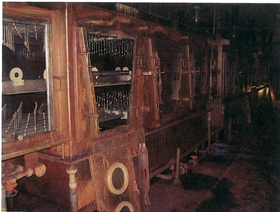
Photograph 16: The pH of the condensation on this process line in Room 5-133 is 3.
