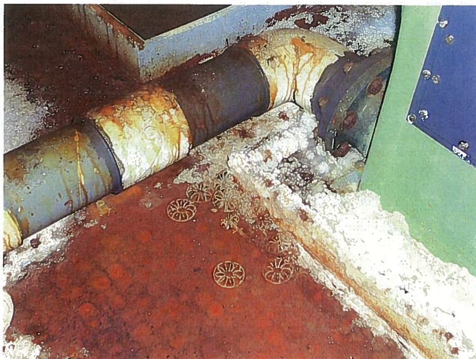
Photograph 10: Sample location 31 (BM-SW-21/BM-SW-22), tellerettes from inside the ventilation system.
