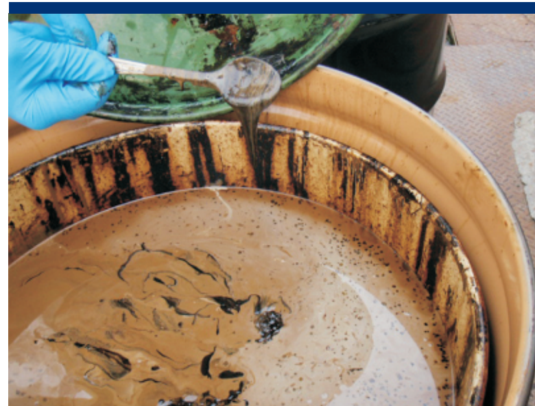
Photo 62 START collecting sample from overpacked drum for hazard categorization.
