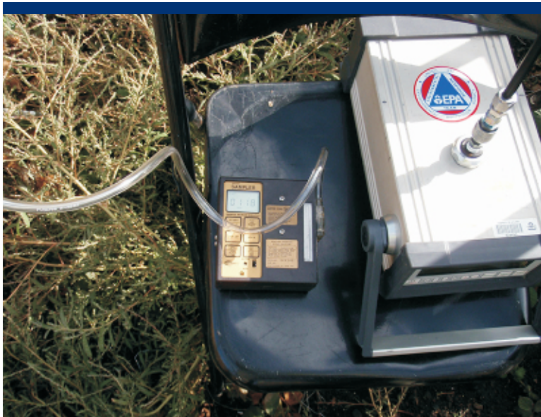
Photo 45 Asbestos and dust sampling equipment.
