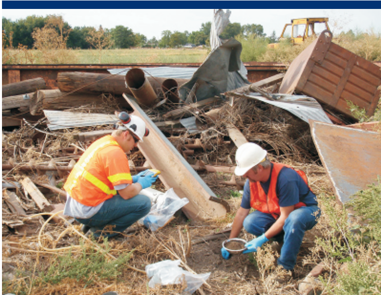
Photo 23 Collecting surface soil samples in the drum field.
