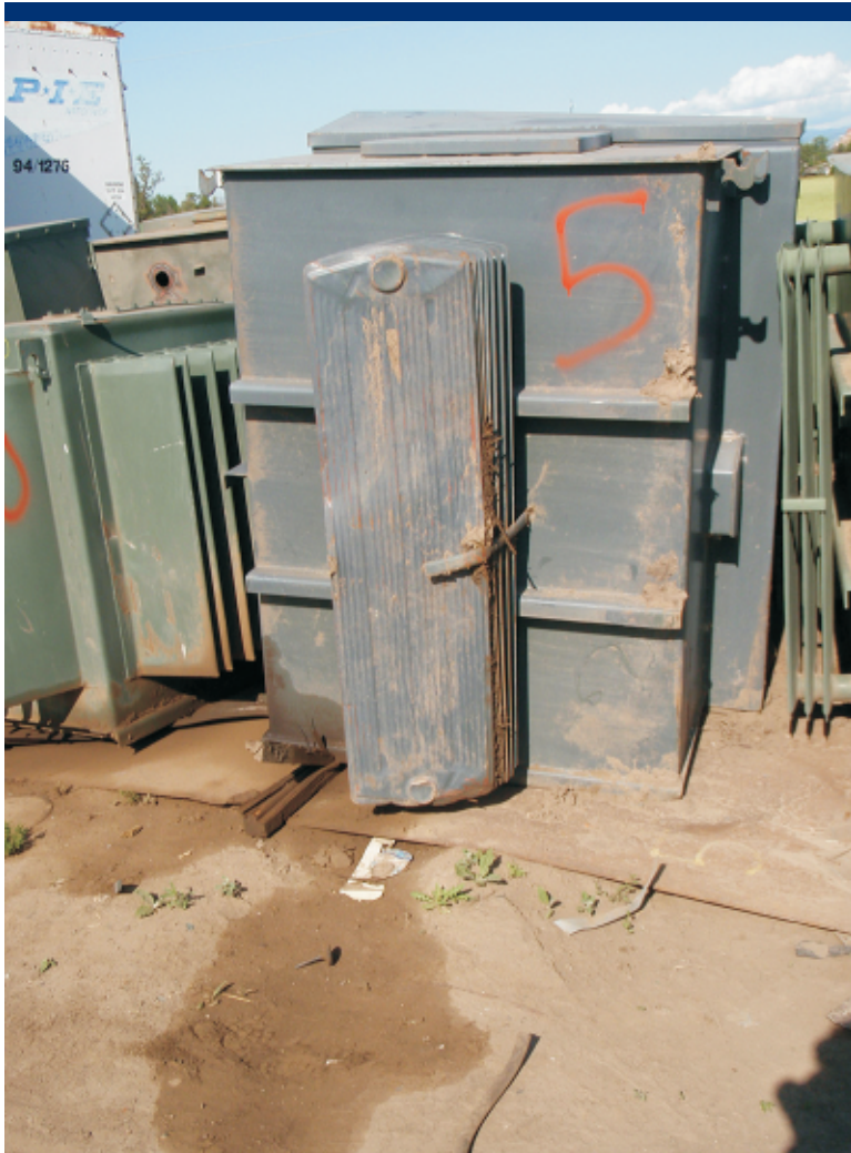
Photo 16 Leaking transformers.
