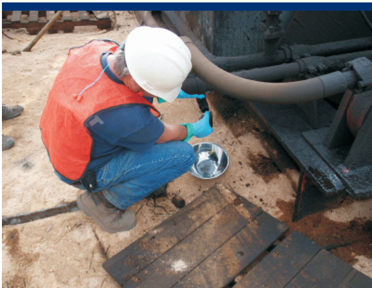
Photo 21 Collecting product samples from hydraulic equipment.
