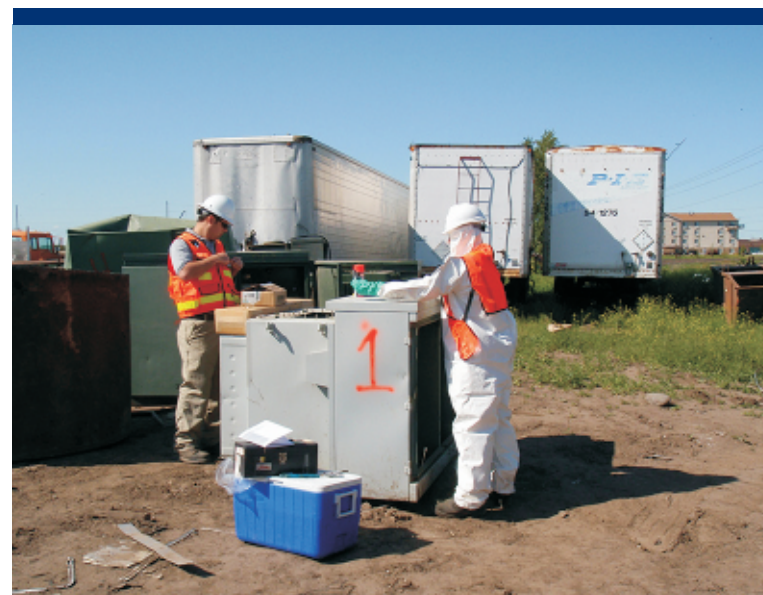
Photo 18 Sampling transformer oil.
