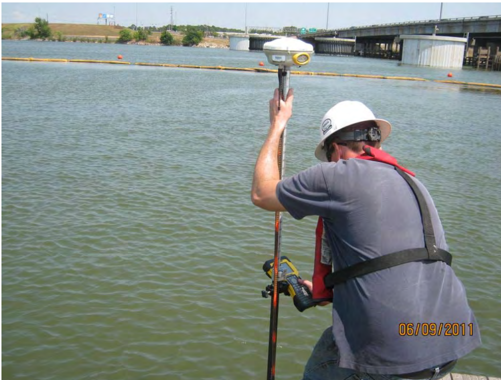
Photo 4 – Collecting survey data for a cap thickness measurement in the Eastern Cell.
