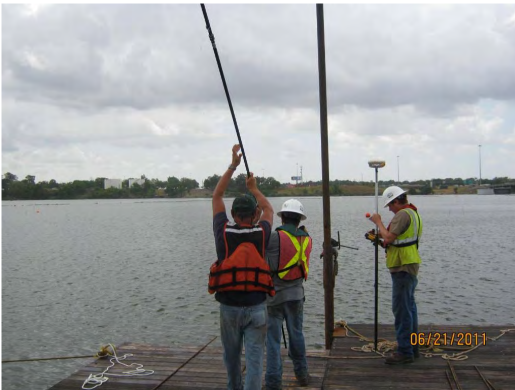
Photo 5 – Collecting Armor Cap B/C cap thickness data in the northwestern area.
