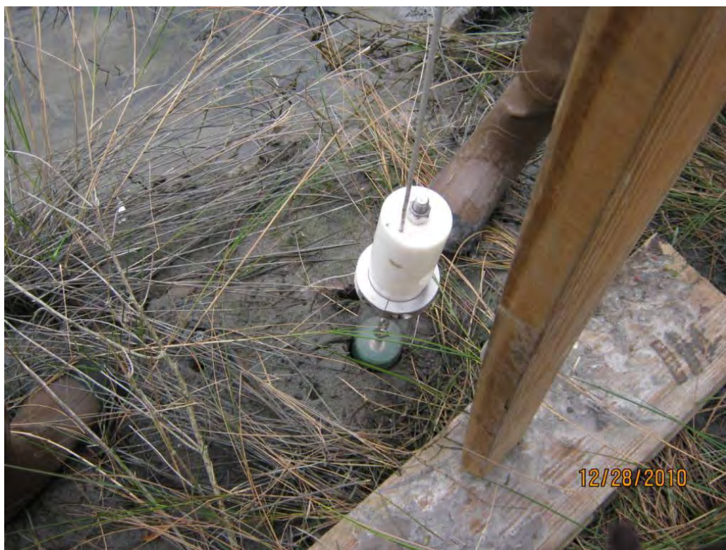
Photo 2 – Piston core sampler advanced at SJPERM03 sample location.
