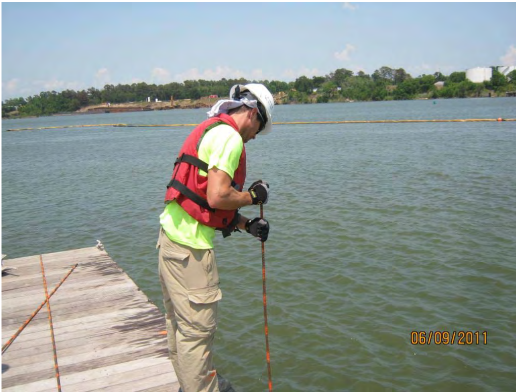
Photo 3 – Using a section of rebar to probe cap thickness in the Eastern Cell.
