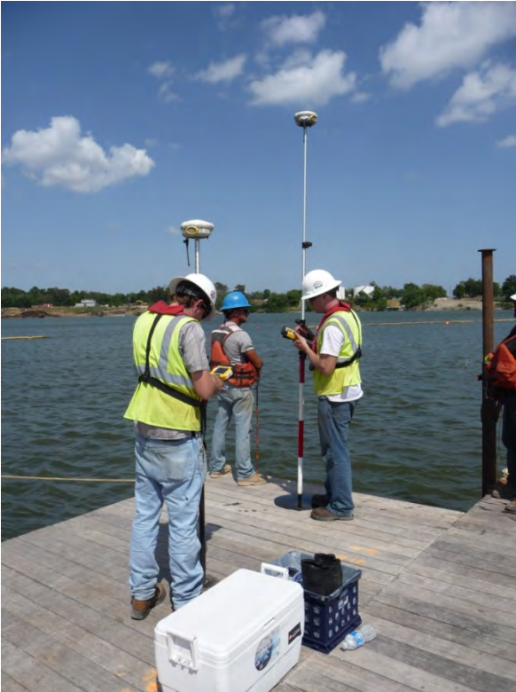
Photo 2 – Survey equipment used to identify and record armored cap thickness points.
