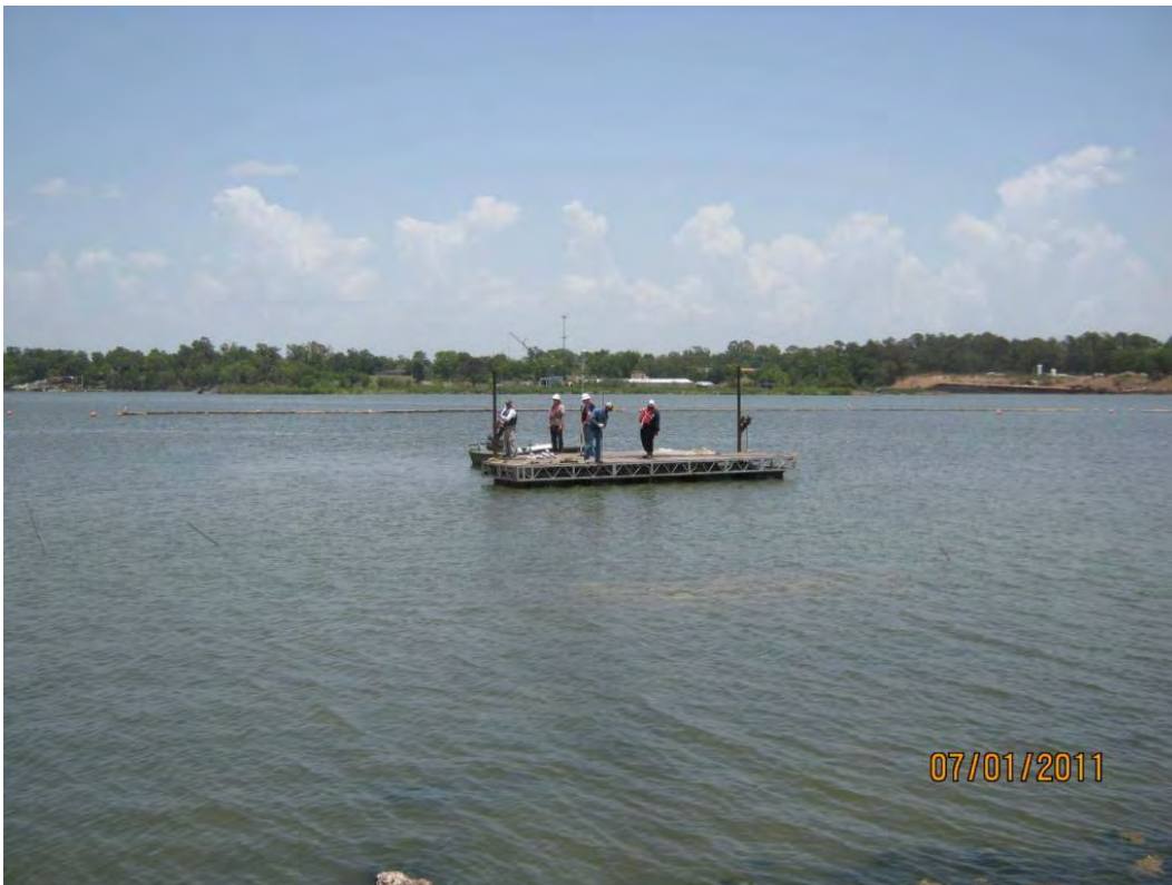
Photo 2 – Collecting armored cap thickness measurements in the Eastern Cell.
