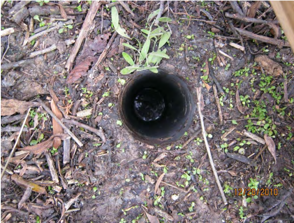
Photo 6 – Open borehole shortly after retrieving sample from SJPERM01 location.
