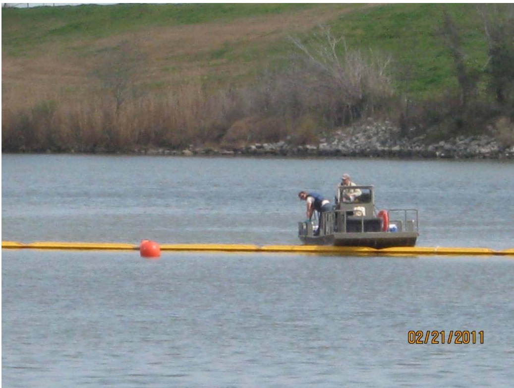
Photo 2 – Collecting turbidity data immediately outside turbidity curtain outside east cell
