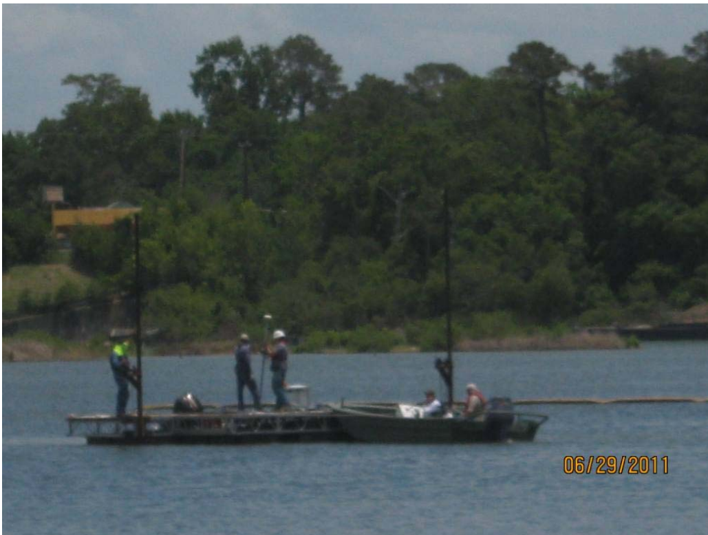
Photo 2 – Collecting armored cap thickness data in the Eastern Cell.
