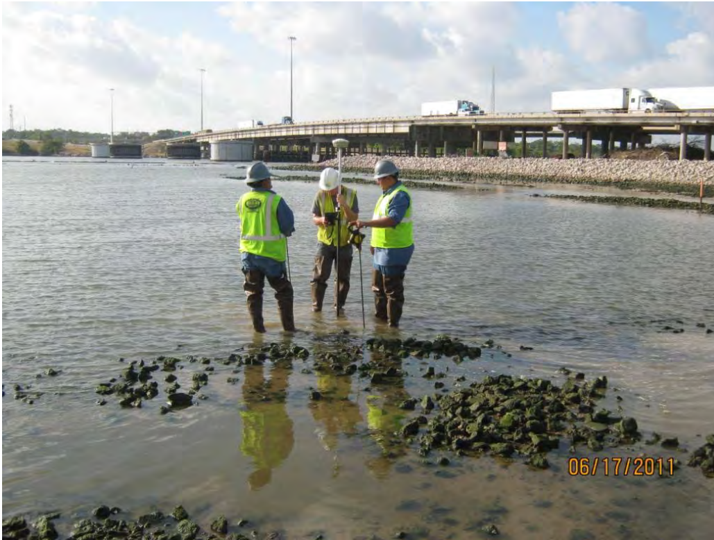
Photo 2 – Survey crew in hip waders measuring armored cap thickness at near-shore areas near low tide.
