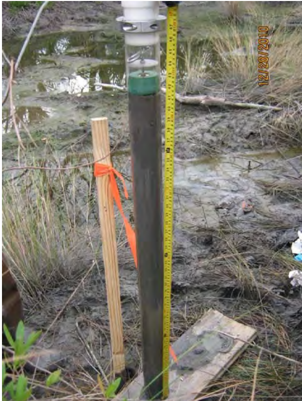
Photo 3 – Core sample collected at SJPERM03 sample location.
