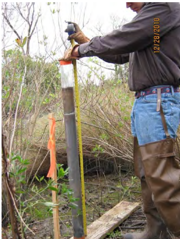
Photo 3 – Core sample collected at SJPERM03 sample location.
