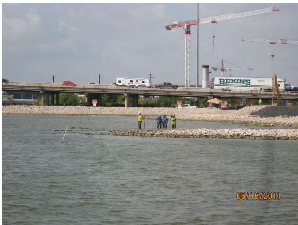
Photo 1 – Armored cap thickness probing using waders in a shallow-water area.
