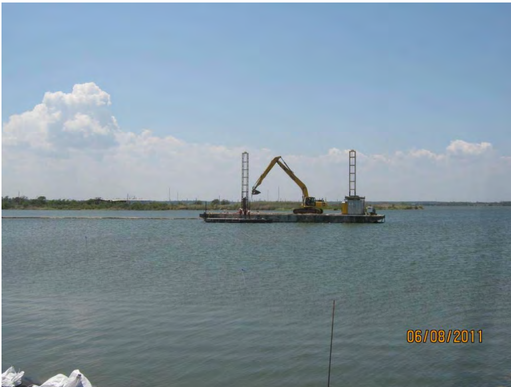
Photo 4 – Preparing geotextile deployment barge for use in collecting cap thickness measurements.
