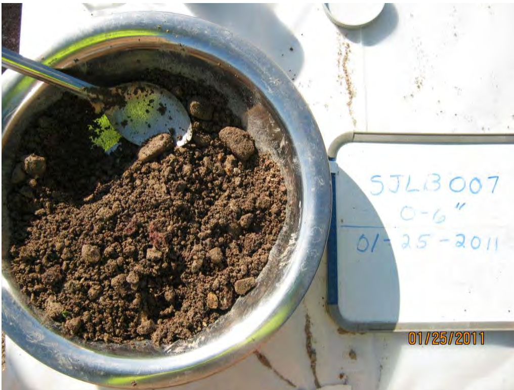
Photo 8. Surface soil sample from SJLB007 location after homogenization, prior to placing into appropriate sample containers
