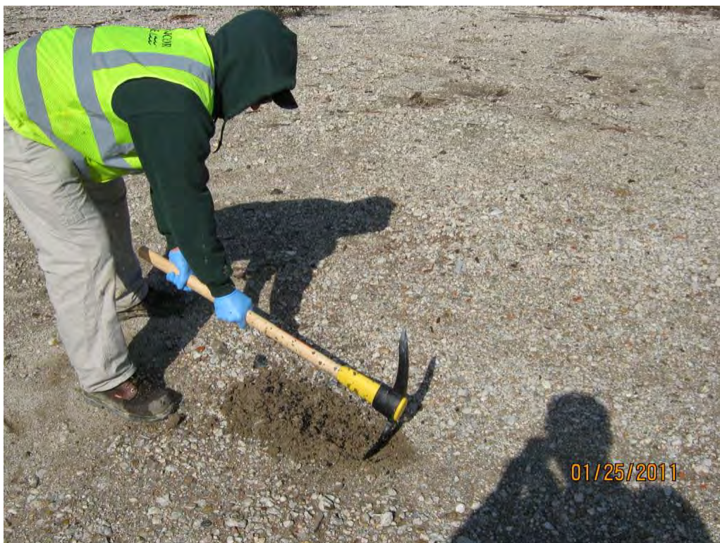
Photo 4. Collecting surface soil sample using pick axe
