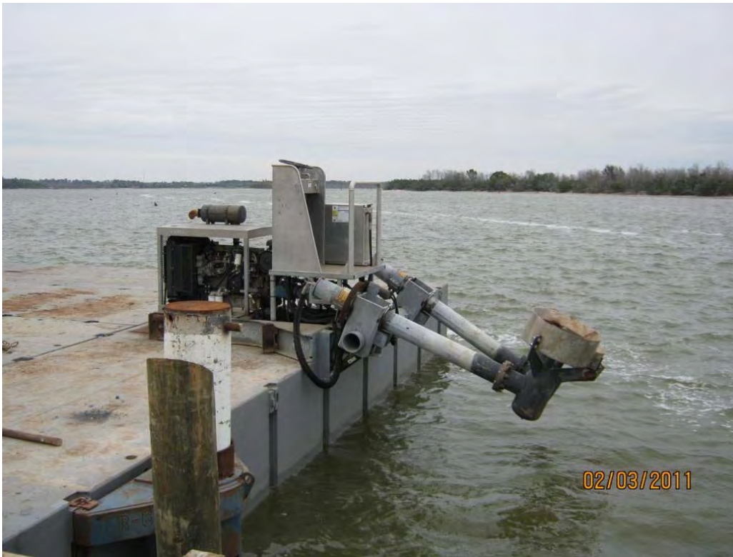
Photo 5 – Motor and propellers mounted onto aggregate transport barge
