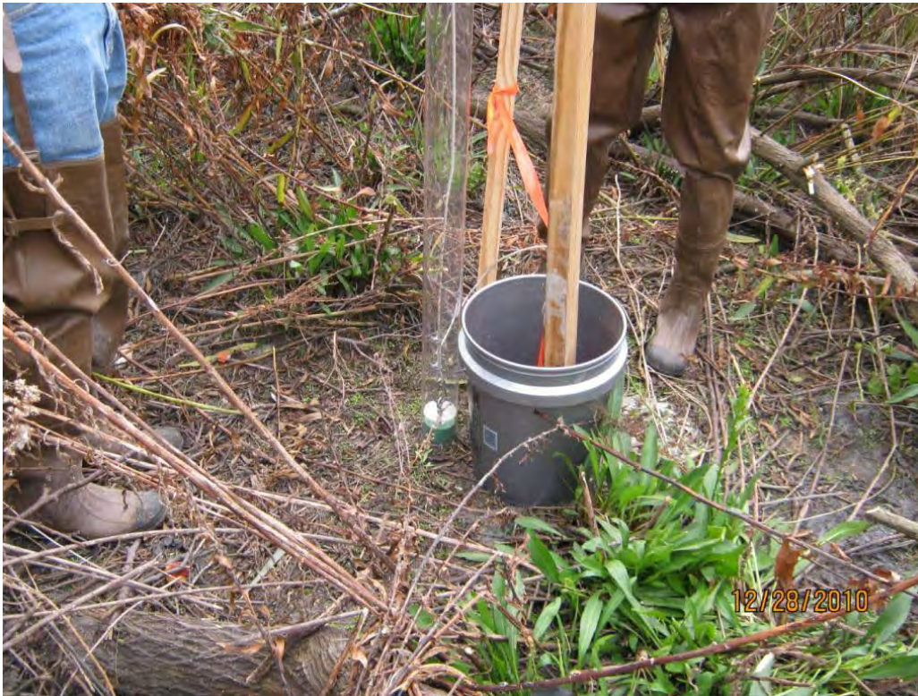
Photo 5 – Collecting core sample from SJPERM01 location.
