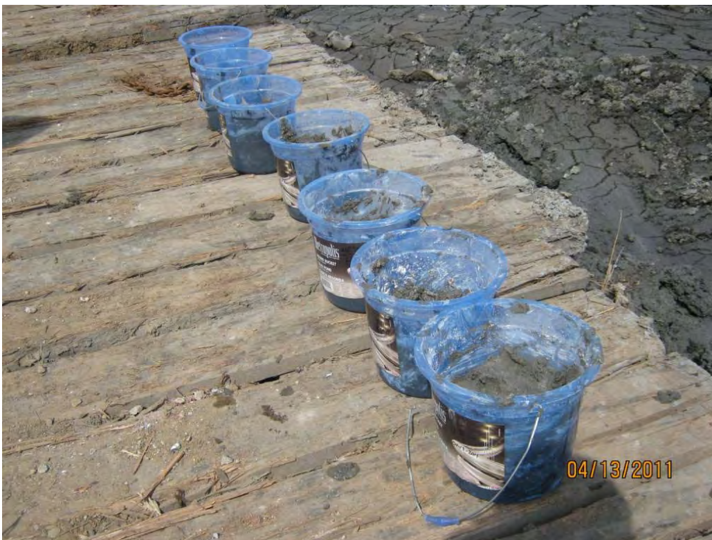
Photo 4 – Sediment stabilization test samples collected from the west cell.
