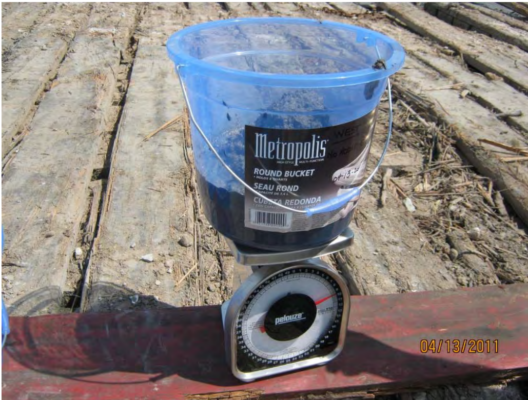
Photo 3 – Weighing a sediment sample for preparation of a sediment stabilization test sample.
