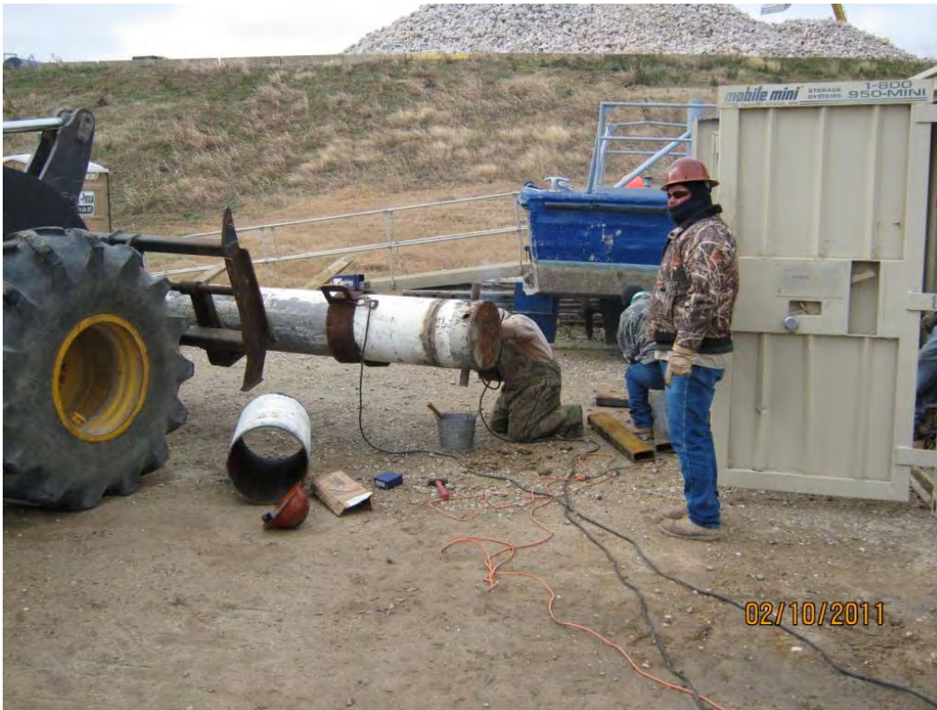
Photo 5 – Weld work on spud for aggregate transport barge
