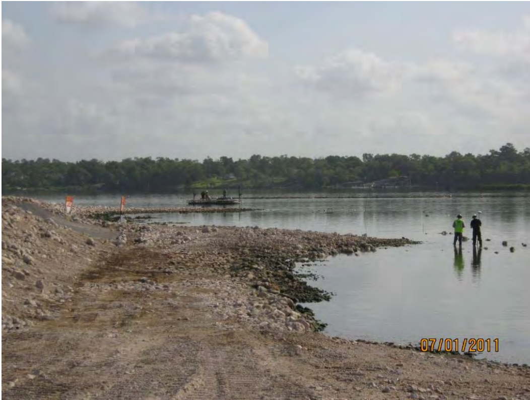
Photo 1 – Collecting armored cap thickness measurements in the Eastern Cell from a dock and using waders.
