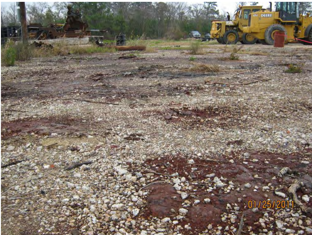
Photo 6. Red surface staining near east corner of upland lease area at LaBarge property; drums (background) have "red resin" labels
