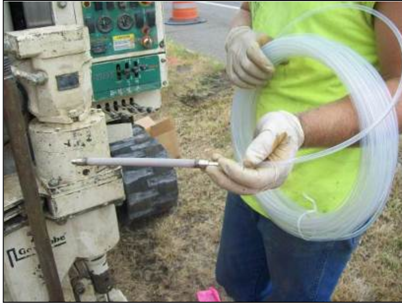
Site: South Dayton Landfill Site Photograph No.: 3 Direction: South Subject: Soil gas probe with Teflon tubing
