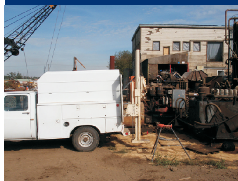
Photo 16 Collecting subsurface soil samples in the west section of the process area.
