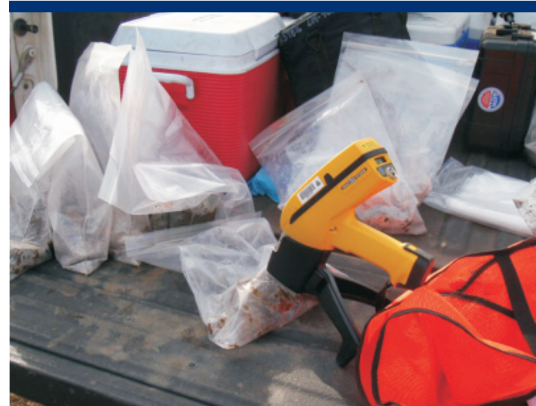
Photo 48 Field screening for metals with XRF instrument.
