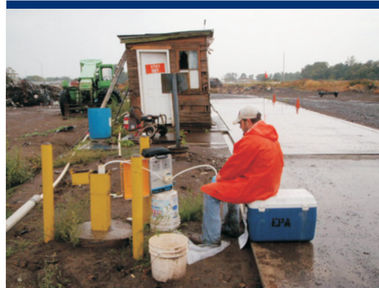
Photo 55 Sampling from monitoring well MW01.
