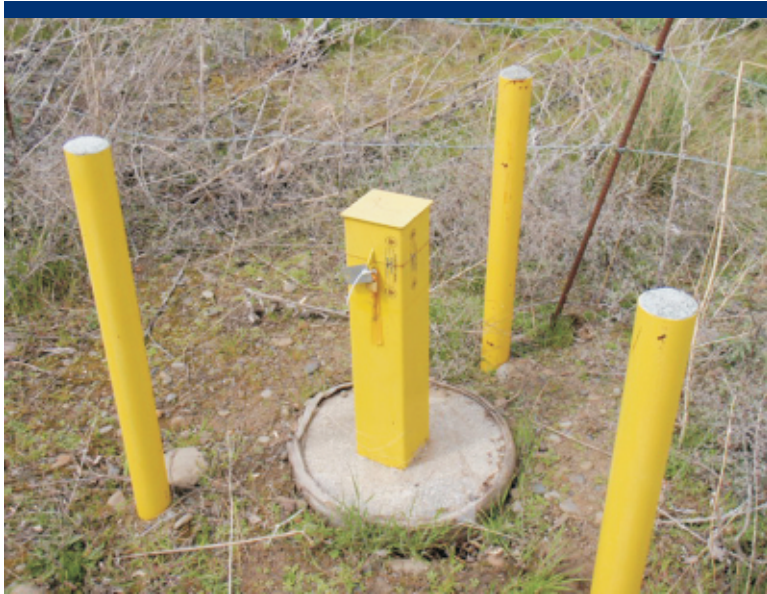
Photo 82 Intact monitoring well MW03.
