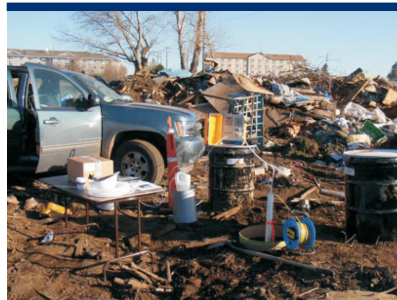
Photo 49 Purging recently installed monitoring well MW04.
