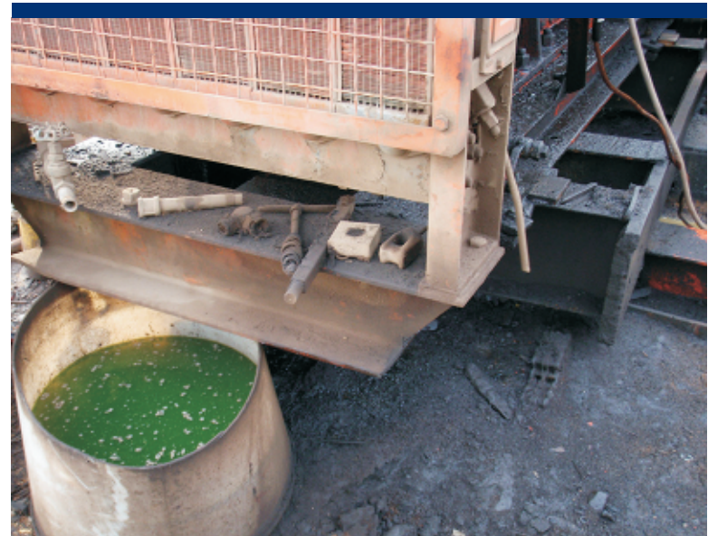
Photo 30 Open container of hydraulic fluid and stained soil by the engine.
