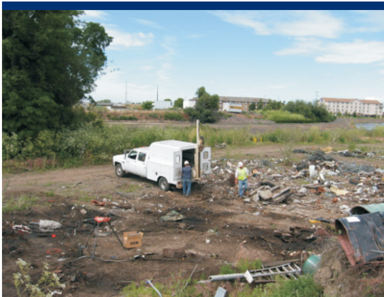
Photo 68 Installing a borehole in the process area.
