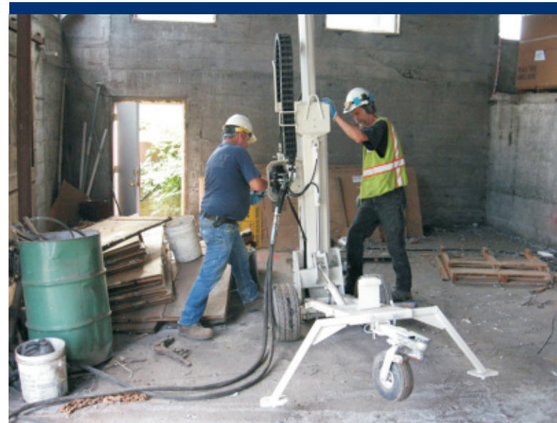
Photo 65 Installing a borehole in soil underneath the shop building.
