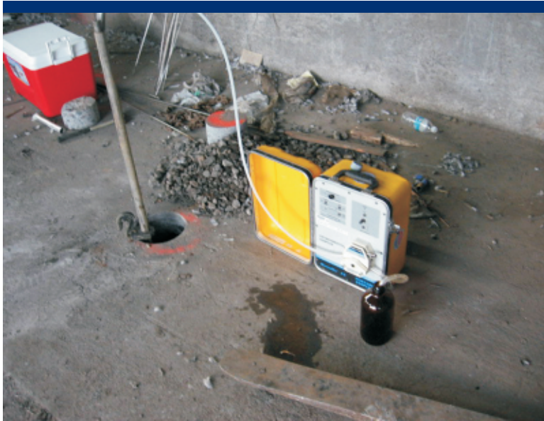
Photo 66 Collecting a groundwater sample from a borehole in the shop building.
