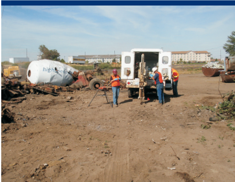
Photo 15 Collecting subsurface soil samples in the process area.
