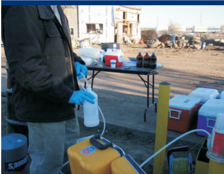
Photo 54 Sampling from monitoring well MW01.
