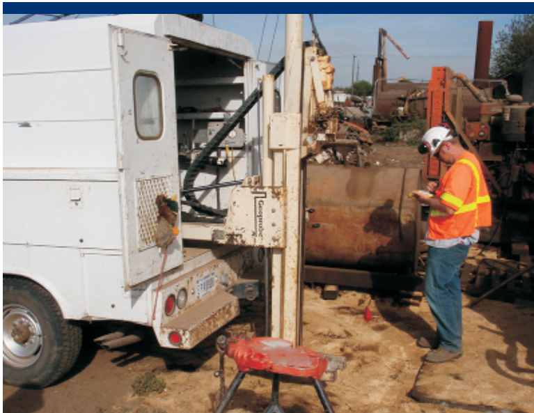
Photo 17 Collecting subsurface soil samples in the west section of the process area.
