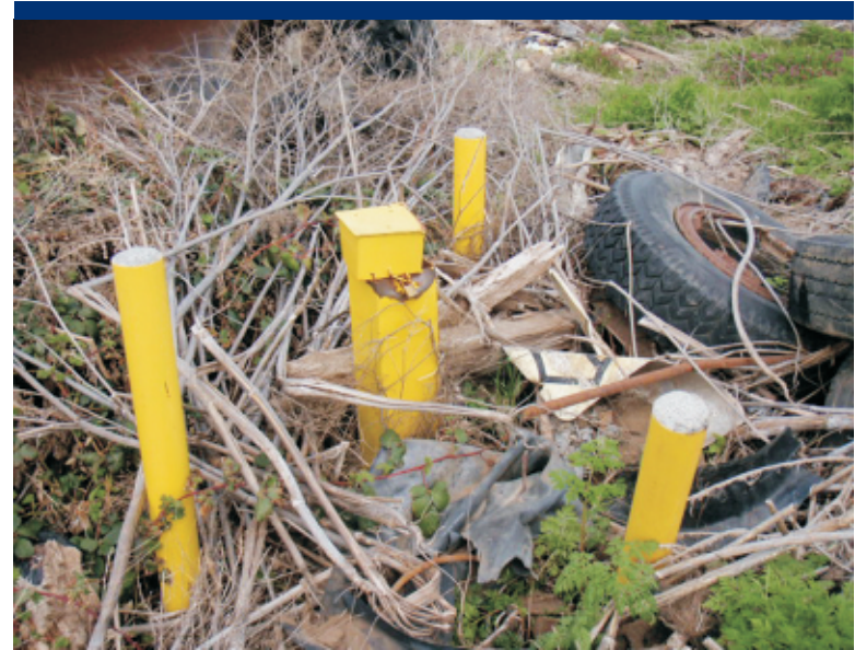
Photo 79 Closeup of damaged monitoring well MW04.
