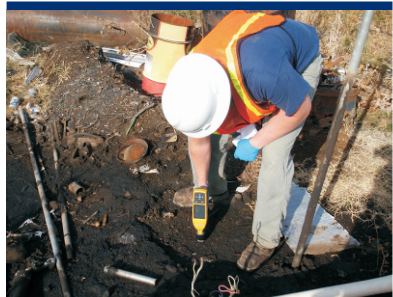
Photo 34 Using an XRF instrument to analyze stained soil for metals.
