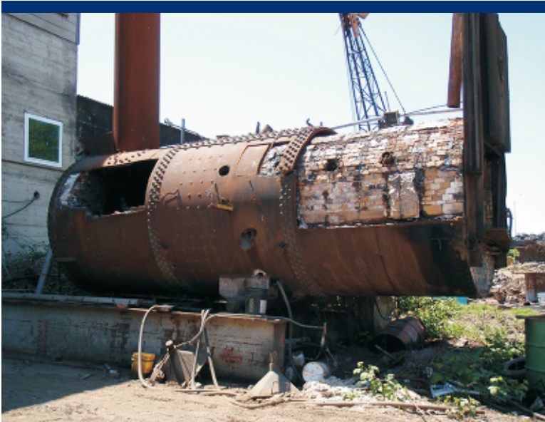
Photo 5 Kiln, reportedly used to melt engine blocks.
