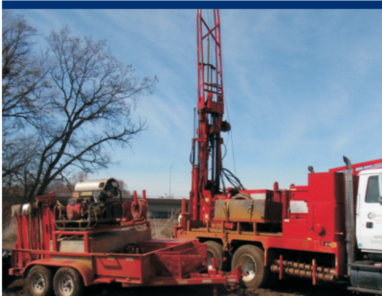
Photo 43 Drill rig setting up at monitoring well MW03.
