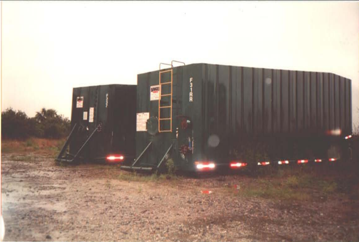
Picture: 13 of 47 Date: 4/7/2005 Time: 2:54 pm Direction: looking SE Agency: Georgia Hazardous Waste Management Branch Photographer: Eddie Williams Subject: View of "frac" tanks on CSX rail property. Tanks were used to store wastewater for future treatment.
