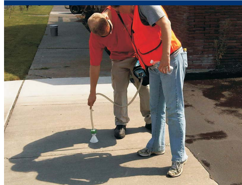
Photo 10 START using Lumex to assess contamination after sealant has been applied.
