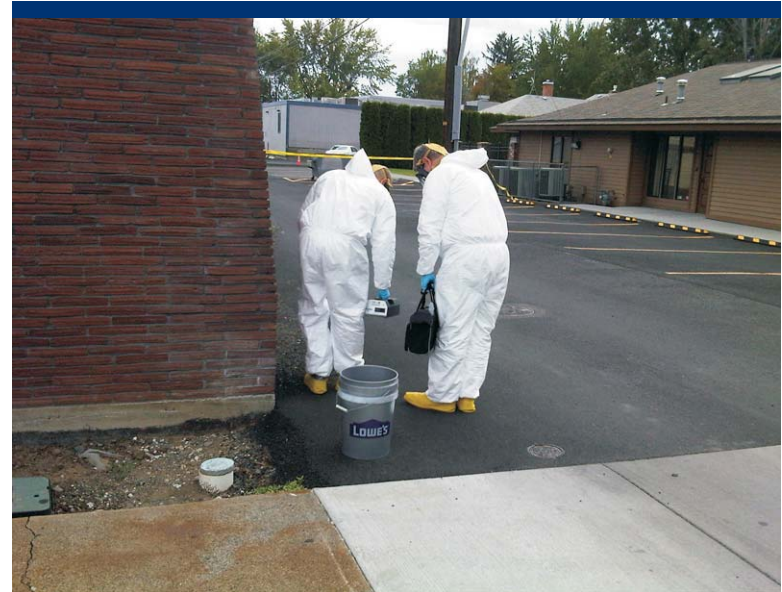
Photo 2 START using the Lumex and Jerome to assess contamination in the exclusion zone
