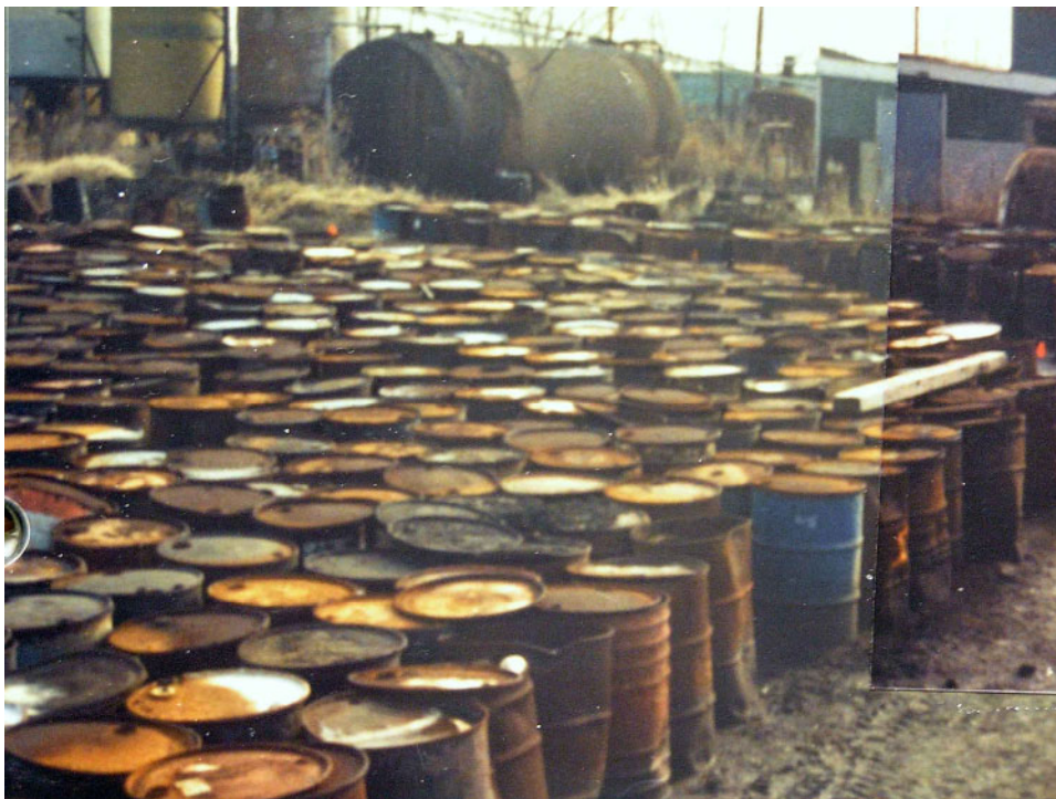
Photo Metro-Trainer.89-15: Close-up view to the southeast of Photo Metro-Trainer.89-14. Note how many of the drum lids were not fully closed, causing sludge to spill out of the drums during precipitation events. Also visible are three acid tanks (far left background), a DAF sludge tank (black tank in center background) and the wastewater treatment plant (right background).
