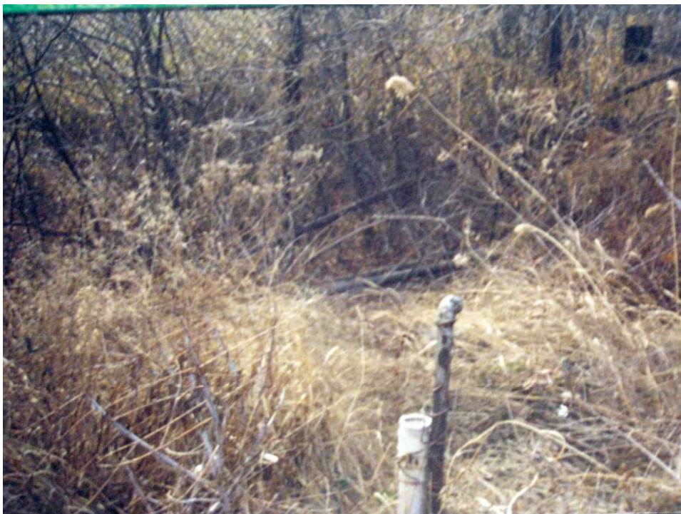
Photo Metro-Trainer.89-27: View to the south of the former MW-6 monitoring well, located on the perimeter of the former disposal lagoon; groundwater impacts were noted as early as 1981 in this and other monitoring wells on the property, but no action was taken to correct the source of the contamination. The security chain-link fence installed by a USEPA subcontractor in September 1988 is visible in the background.
