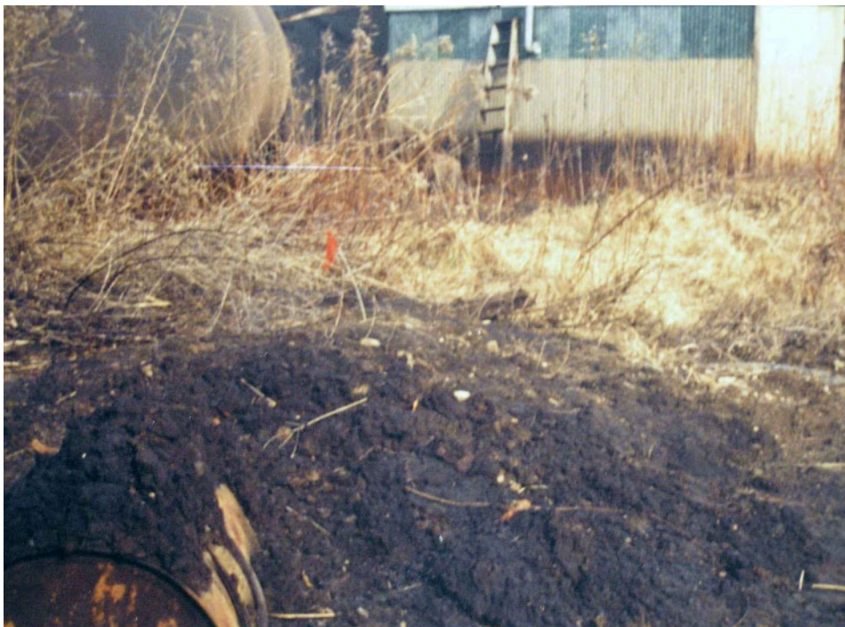
Photo Metro-Trainer.89-25: Close-up view to the northeast of the berm of the secondary containment impoundment depicted in Photo Metro-Trainer.89-22; note the partially buried drum in the left foreground. Buried drums, used as fill, were discovered in the 2005 Site Characterization underlying the northwestern corner of the property.
