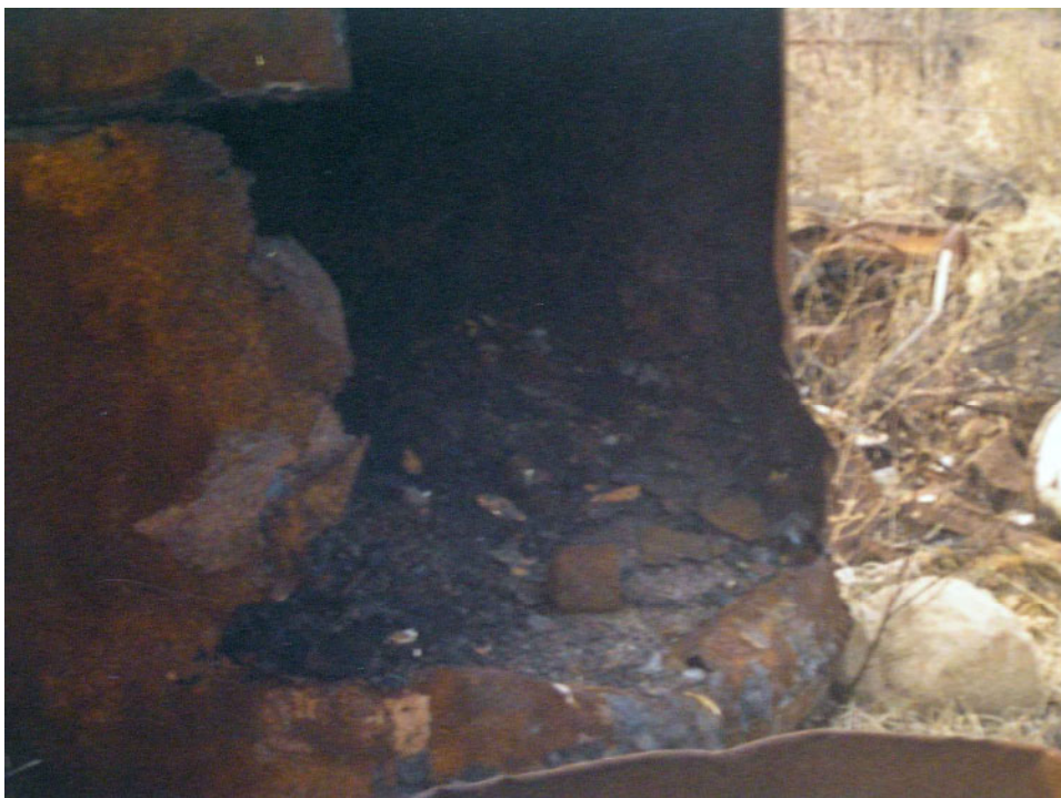
Photo Metro-Trainer.89-26: Close-up view to the southeast of the incinerator at Metro Container Corporation site. This may have been part of the furnace treatment process (essentially thermal neutralization) that was utilized to remove the exterior paint on the drums and also to prepare unsalvageable drums and buckets for the scrap metal market.
