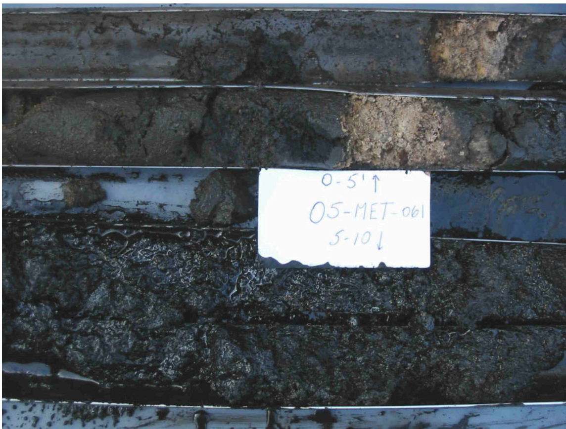
Photo Metro-Trainer.044: Close-up view of the center section of the Geoprobe ® soil cores extracted from the 05-MET-061 location at the Trainer Industries, LLC/former Metro Container Corporation Site. The 5-10 ft bgs interval, comprised of anthropogenic gravel and slag, was saturated with non-aqueous phase liquids (NAPL), seen here seeping into the cardboard identification label.
