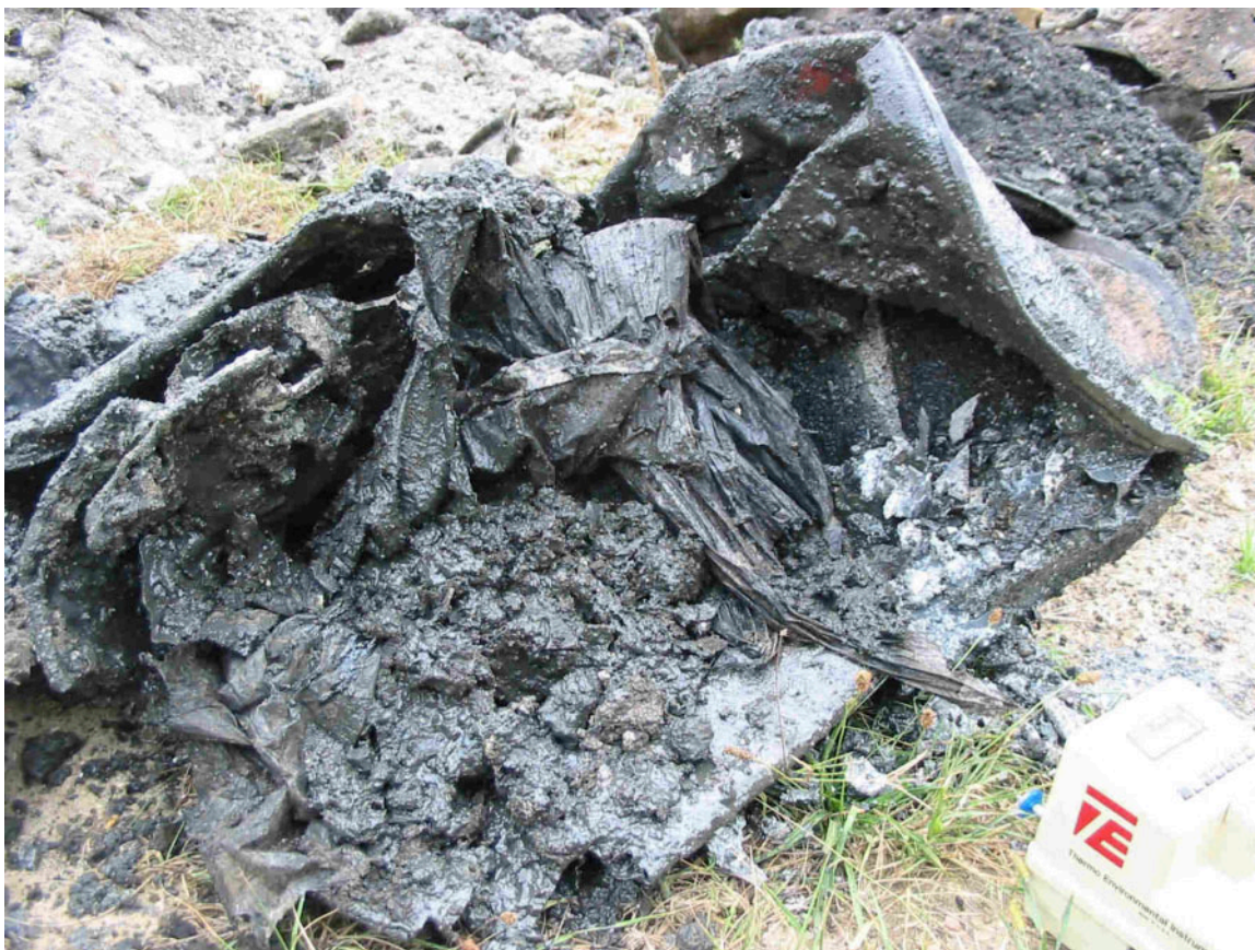
Photo Metro-Trainer.055: View of a crushed 55-gallon removed from the Test Trench-01 excavation at the Trainer Industries, LLC/former Metro Container Corporation site. Many of the crushed drums that were encountered contained small amounts of residual solids that registered PID readings up to 427 ppm. Plastic sheeting was also encountered intertwined with the drums.
