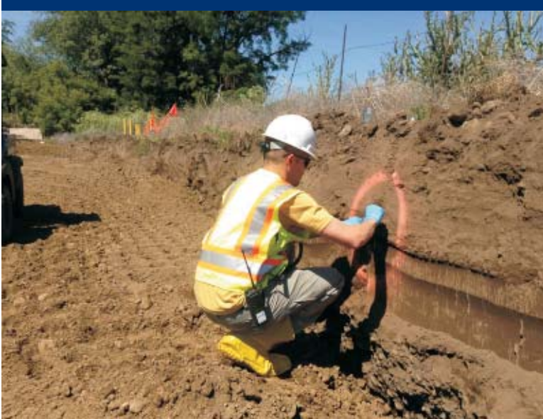
Photo 53 Collecting sidewall soil sample in the NPA with MW3 in the background.
