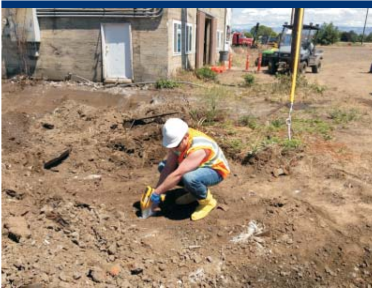
Photo 77 Performing in-situ screening with the XRF of near surface soils in the Upland Area.
