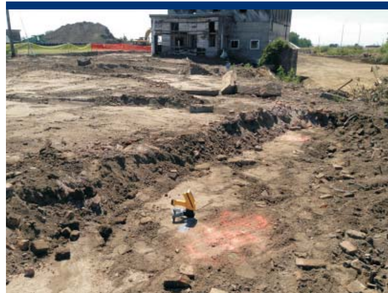
Photo 88 Performing confirmation in-situ screening with the XRF in OU3 in the Upland Area.
