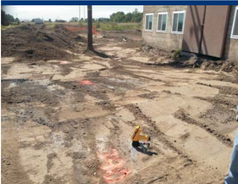
Photo 89 Performing confirmation in-situ XRF screening of discolored soil in OU1 in the Upland Area.
