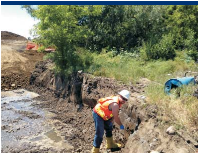
Photo 47 Collecting sidewall soil sample in the northern lobe near the swale.
