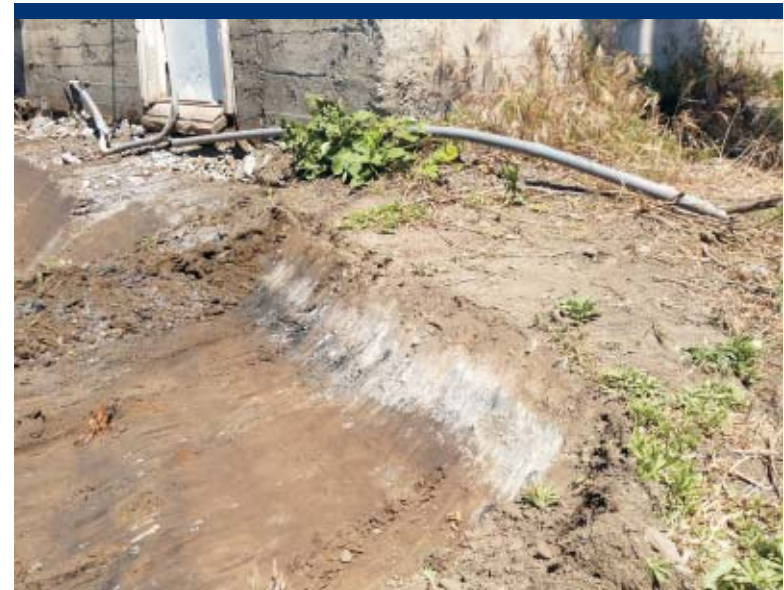
Photo 76 Grey lense of lead-contaminated soil in the Upland Area.
