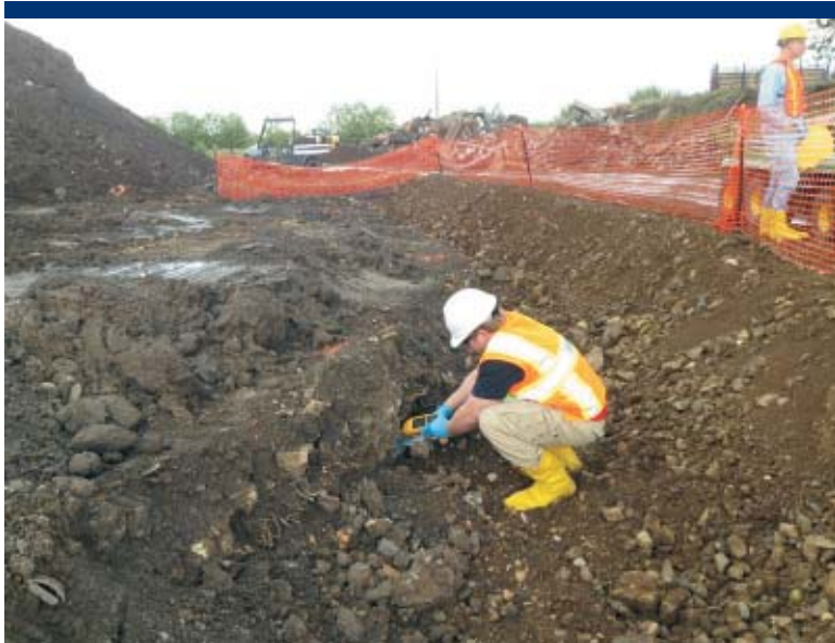
Photo 37 START performing XRF screening of suspected lead-contaminated soil in the Process Area.
