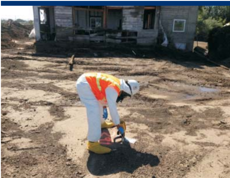
Photo 83 Performing confirmation in-situ screening with the XRF in OU2 in the Upland Area.
