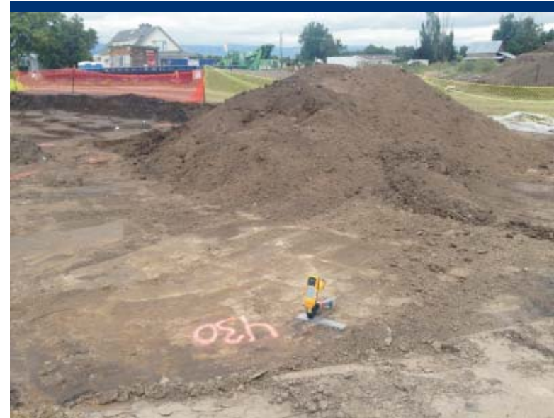
Photo 90 Performing confirmation in-situ XRF screening around the OU1 stockpile in the Upland Area.
