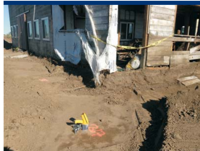
Photo 84 Performing confirmation in-situ screening with the XRF in OU1 in the Upland Area.
