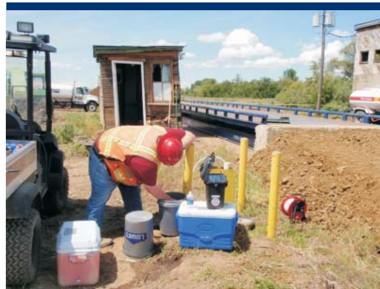
Photo 8 EPA task monitor collecting groundwater sample from MW1.
