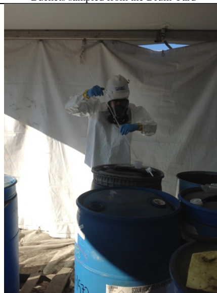
START sampling thawed and cut open drums in Level C PPE
