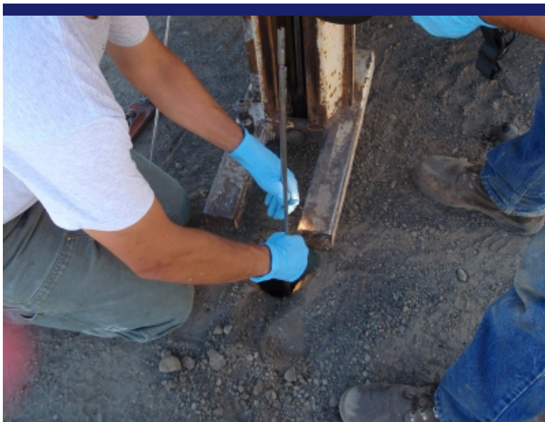
Photo 11 Using flashlight to see down into boring BP12.
