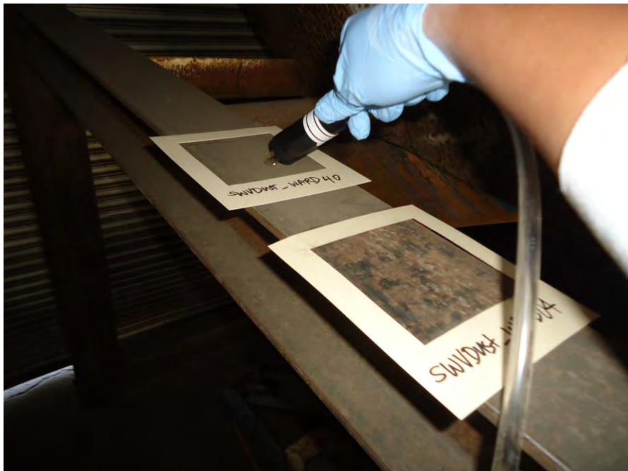
Photograph DSC00776: View looking northeast at "Dust Sampling" of Locations WARD04 and WARD40 (Duplicate), located on a steel cross beam of a Hopper in the north central portion of the main warehouse.
