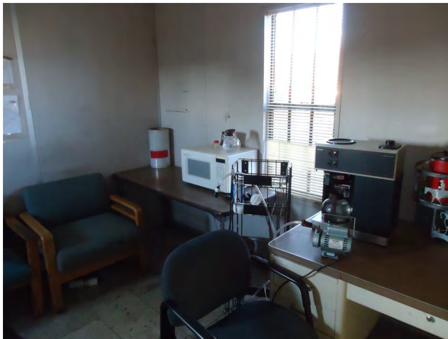
Photograph DSC00963: View looking northwest within the W. Silver Scale House trailer at the Air Sample being collected near the location of recent dust samples with elevated levels of Libby Amphibole.
