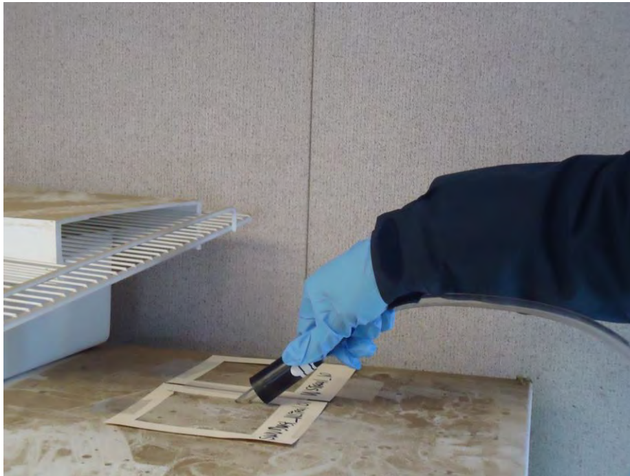
Photograph DSC00869: View looking south within the W. Silver Scale Trailer at Dust Sampling being conducted on top of the break room refrigerator.
