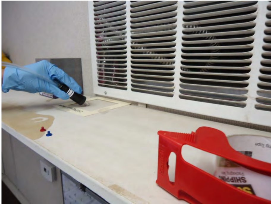
Photograph DSC00951: View looking southeast within the EPA Office Trailer at Dust sampling being collected to assess/confirm the trailer decontamination activities conducted the prior week.
