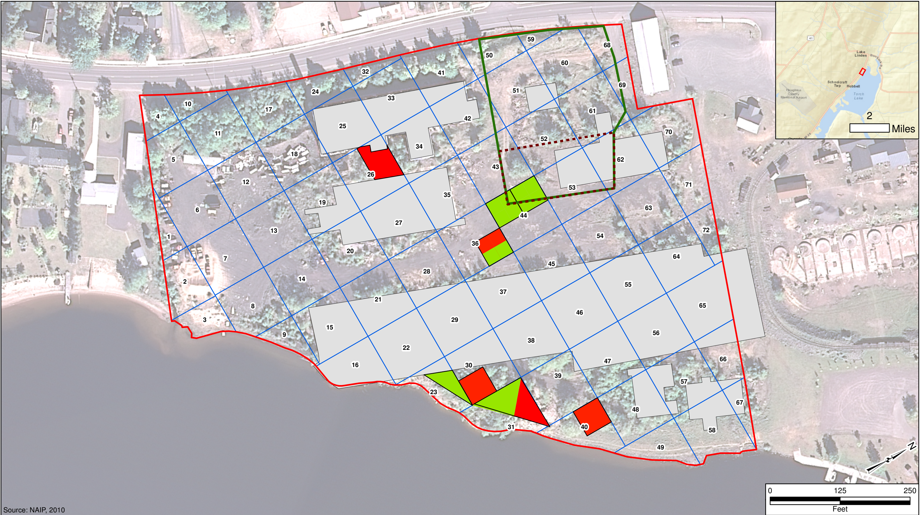
Figure - 2.2 Metals Concentrations Exceeding Non-Residential Direct Contact Criteria Shallow Interval (0' - 0.5') Former C & H POWER PLANT SITE TORCH LAKE TWP, MICHIGAN Project 3293-11-1440
