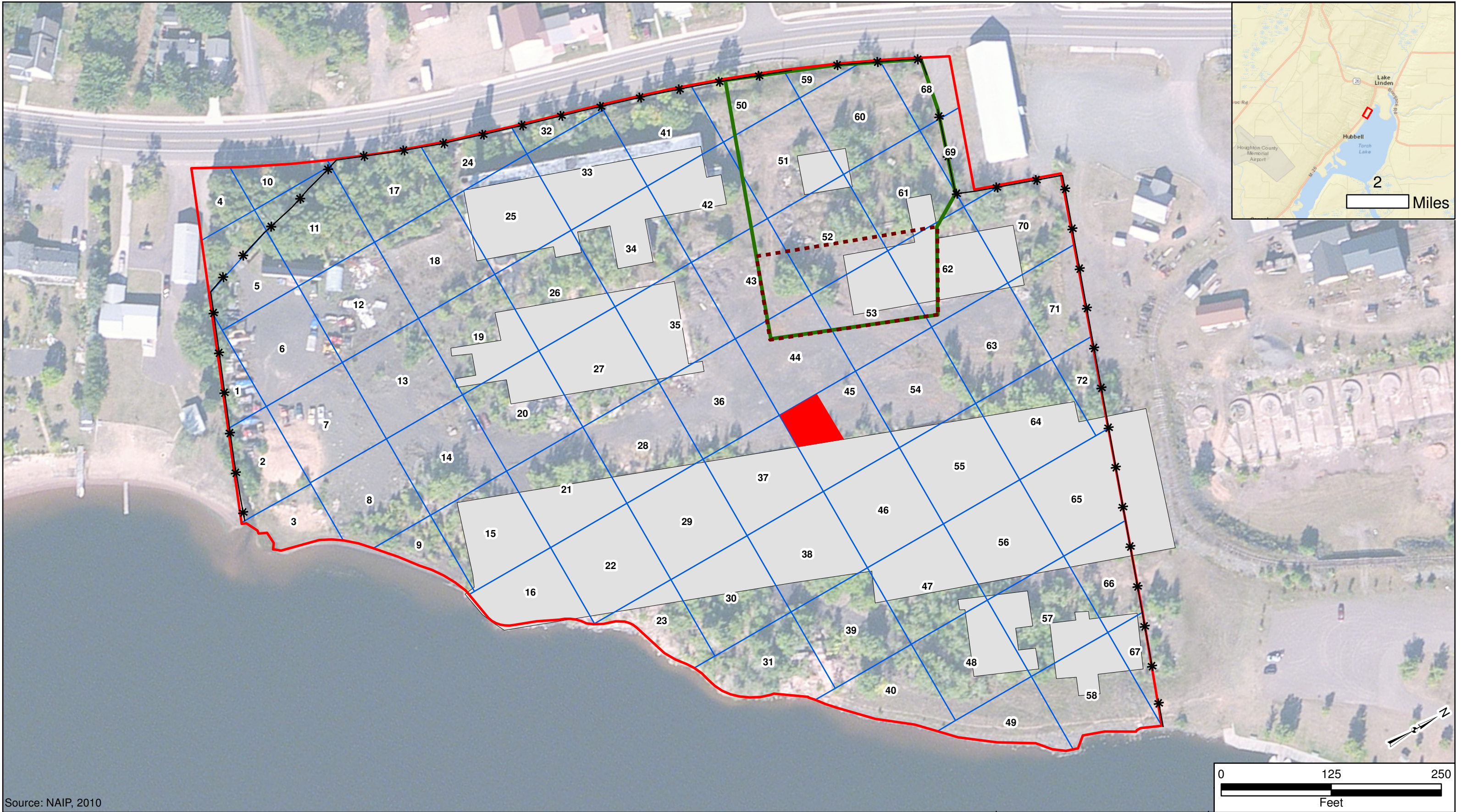
Figure - 2.6 2014 Metals Concentrations Exceeding Non-Residential Direct Contact Criteria Shallow Interval (0' - 0.5') Former C & H POWER PLANT SITE TORCH LAKE TWP, MICHIGAN Project 3293-11-1440
