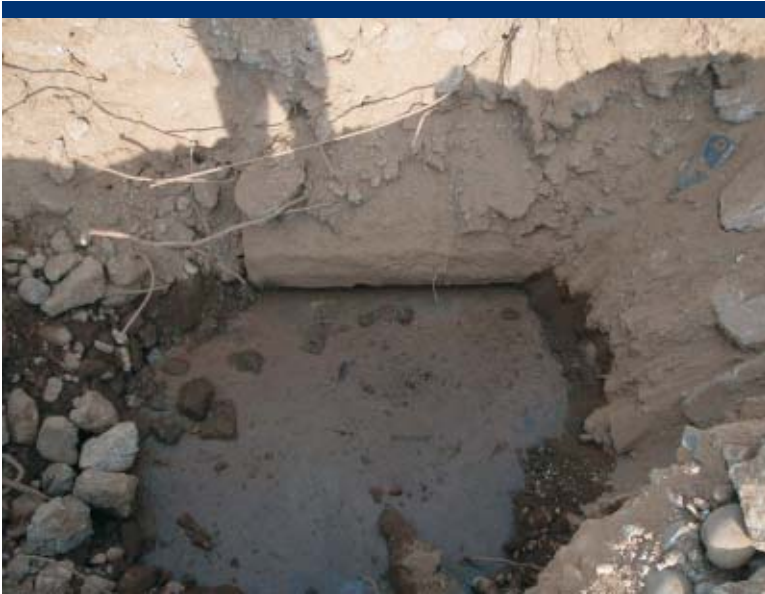
Photo 19 Groundwater at bottom of test pit in southwest quadrant.
