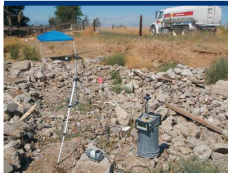
Photo 13 Fill area air sampler FA-01 in northwest quadrant.
