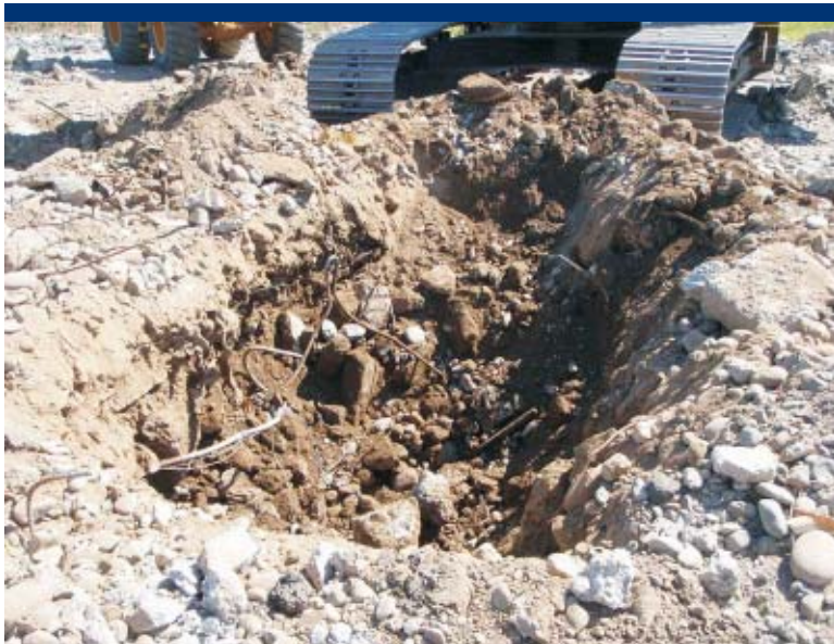
Photo 17 Interior of test pit in northwest quadrant, with river rock, concrete, rebar, and wire.
