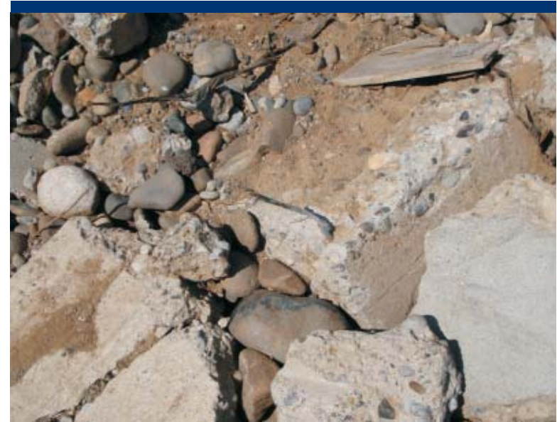
Photo 16 Close-up of concrete in debris pile, with wire and other trash.
