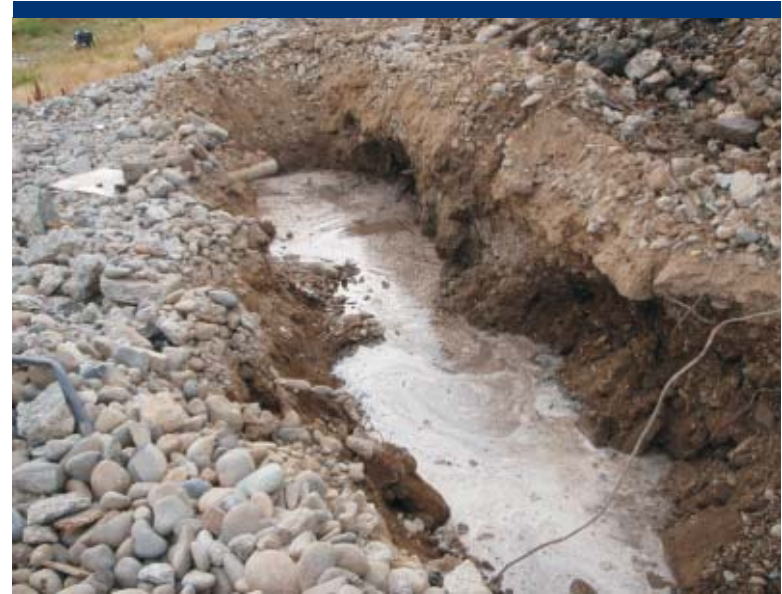
Photo 20 Groundwater in test trench in southwest quadrant.
