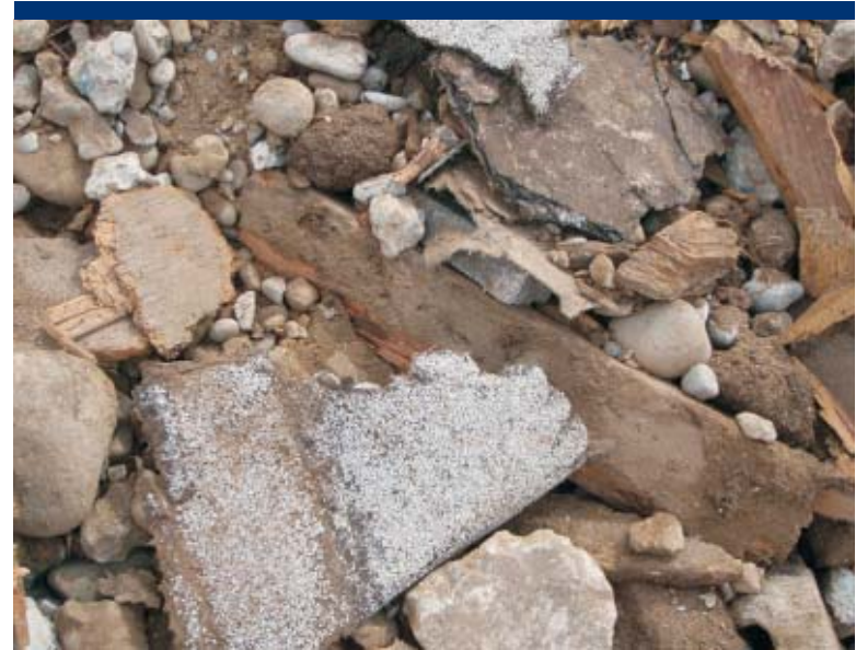
Photo 24 Close-up of roofing material recovered from trench in northeast quadrant.
