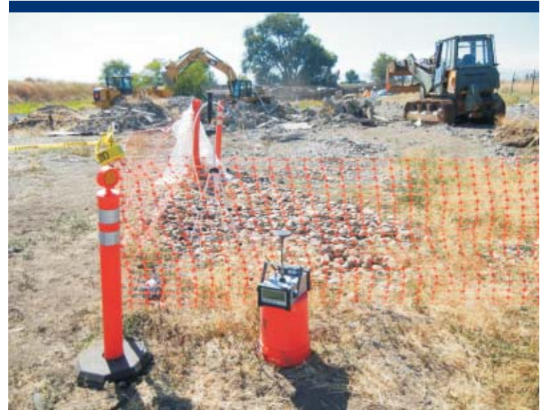
Photo 10 Perimeter air sampler PR01 and DataRAM dust monitor at boundary of exclusion zone near the CRZ.
