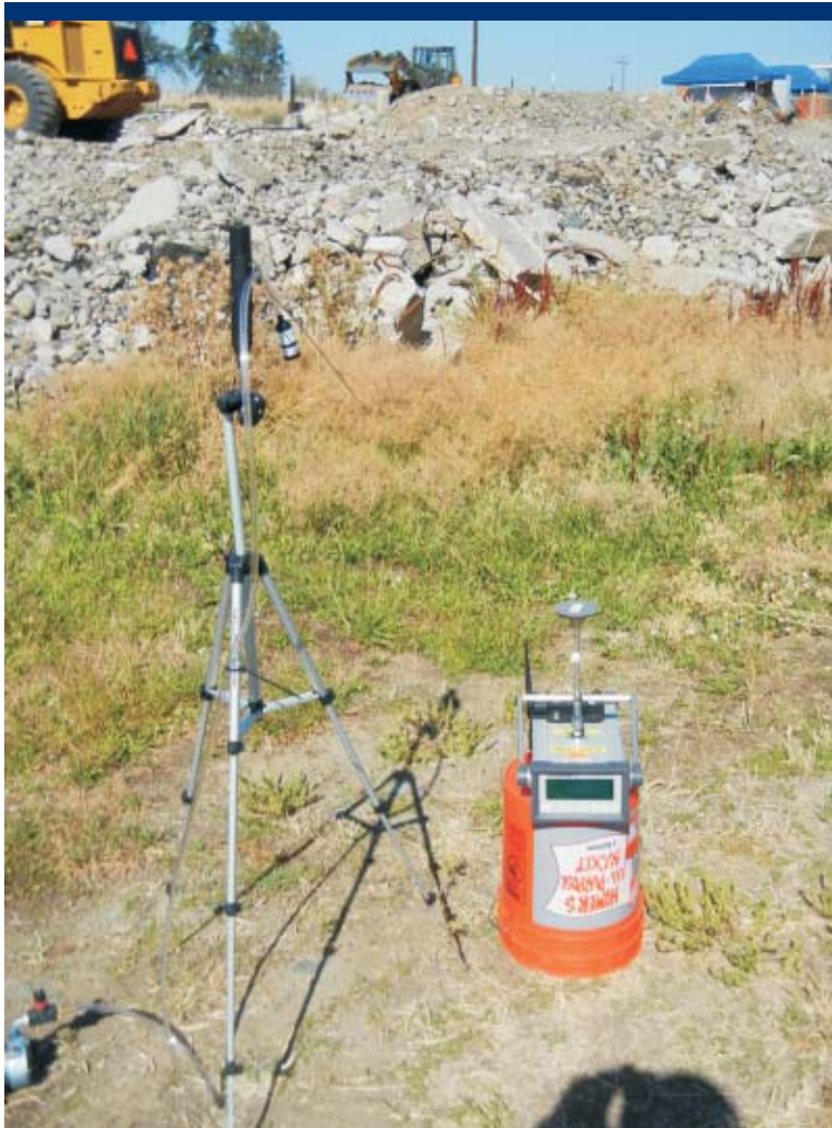
Photo 12 Close-up of air sampler (PR02) and DataRAM dust monitor near southwest corner of debris pile.
