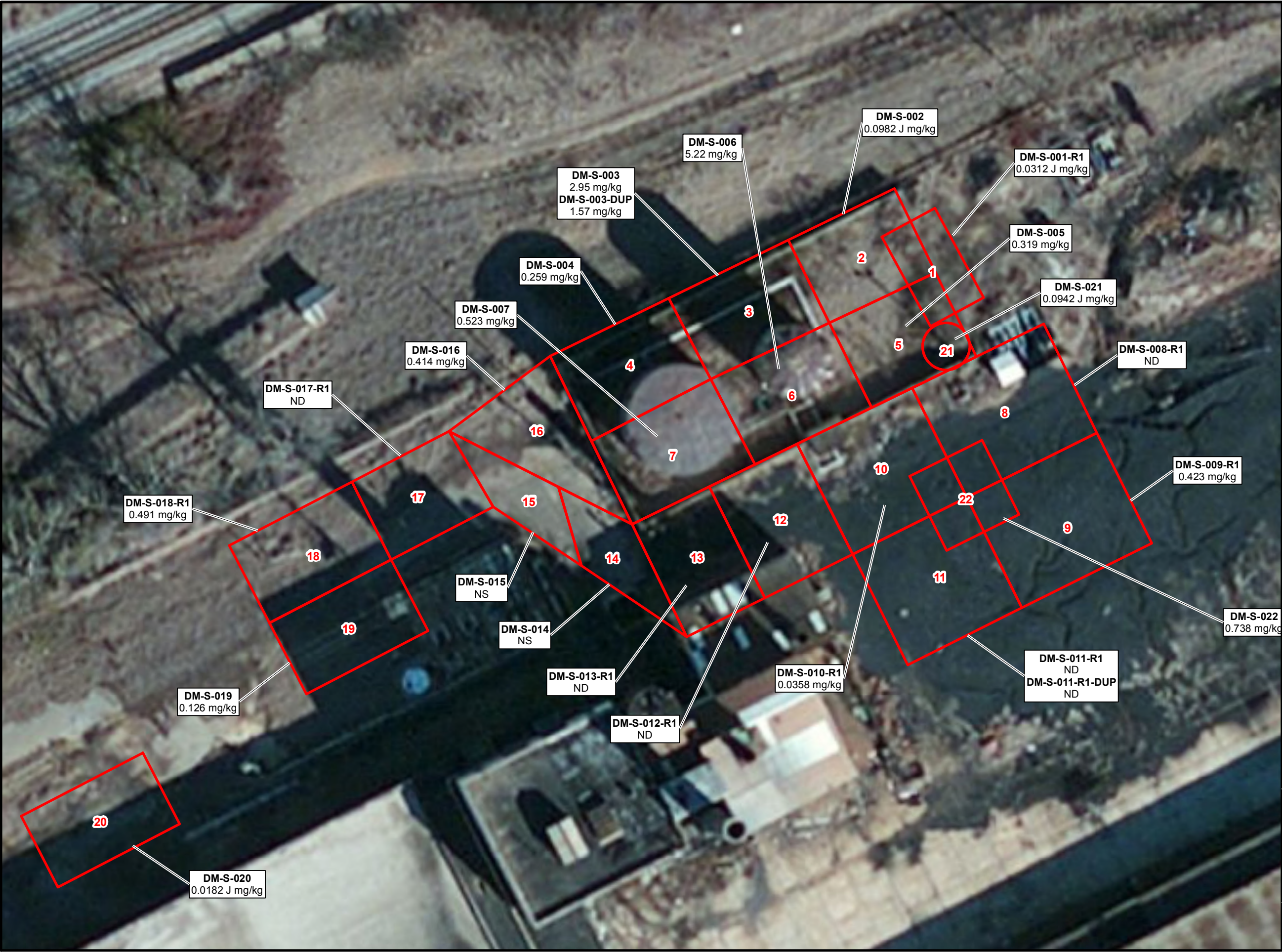
FIGURE 6 Soil Sample Locations and Total PCB Results: Post Excavation and Prior to Backfilling
