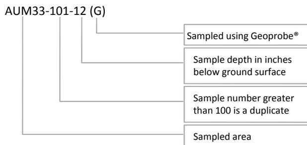
The waste pile (WP) samples were all collected from the surface (0 to 2 inches below ground surface). The last 2 digits of the sample ID of the WP samples represent the sample number.
