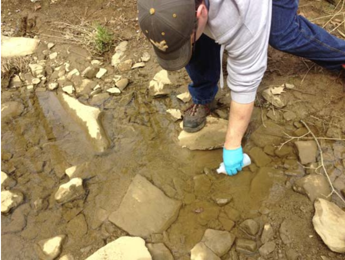
Photo No. IMG_2713; Taken on 03/24/15 at 14:23 hours by START-JW. Facing Down. START team member collecting sample WG-SW-04 by collecting surface water in a dedicated clean sample jar and purging it into the sample bottles.
