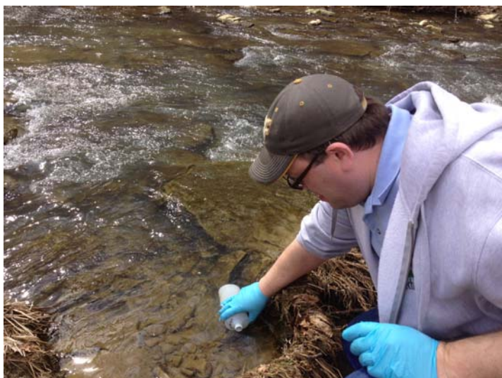
Photo No. IMG_2711; Taken on 03/24/15 at 14:16 hours by START-JW. Facing Down. START team member collecting sample WG-SW-02 and duplicate sample WG-SW-03
