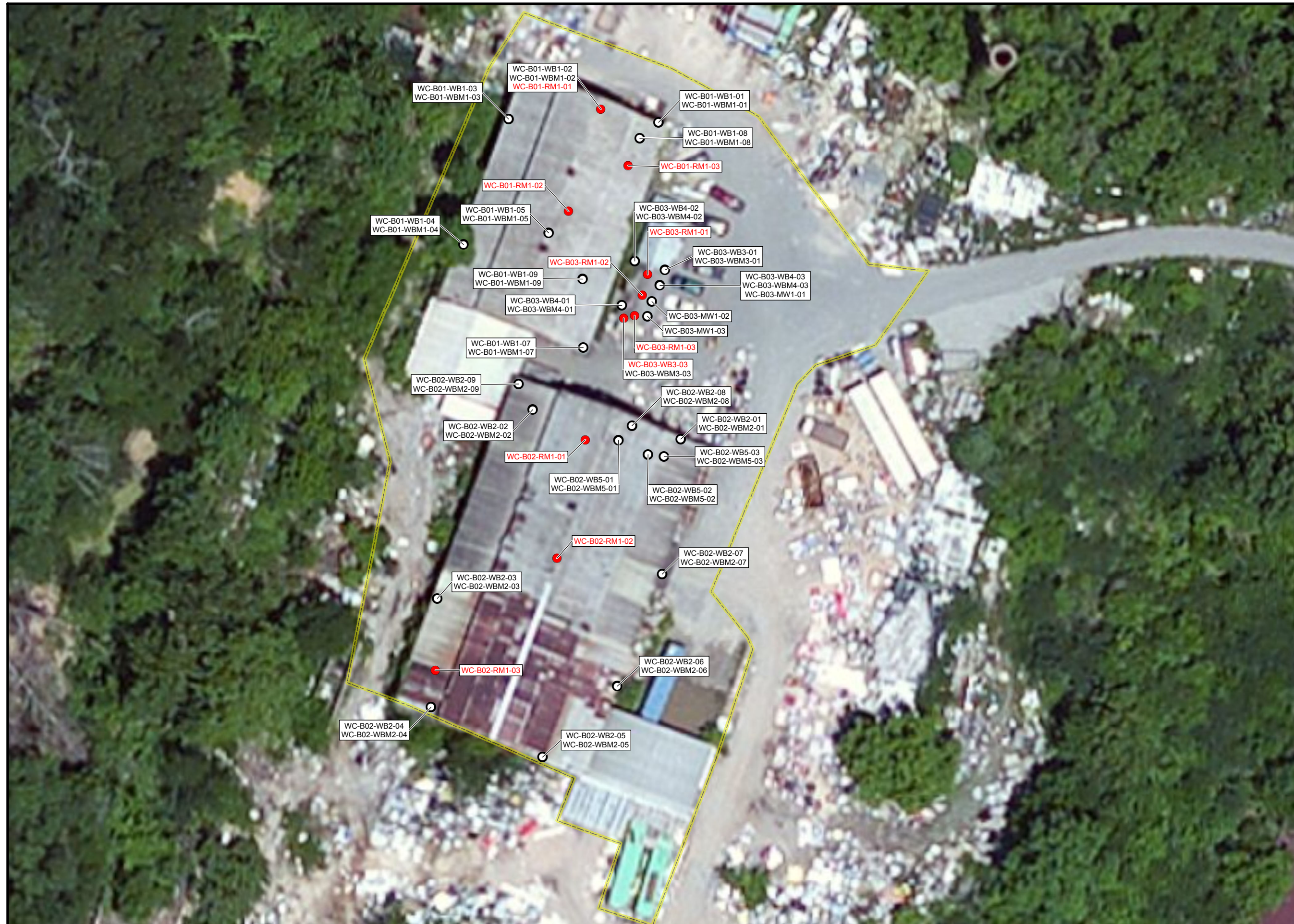
FIGURE 3 Asbestos Bulk Sampling Locations and Results
