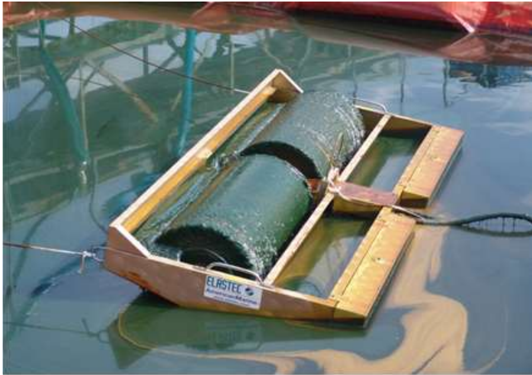
Photo 3 - Photograph of drum skimmer for product recovery.
