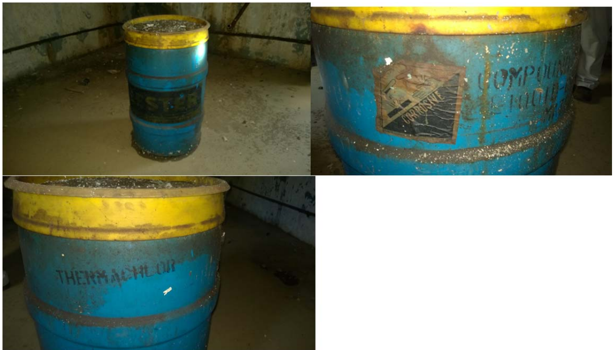
One 55-gallon container in the basement. Corrosive label. Label Information: Thermachlor
