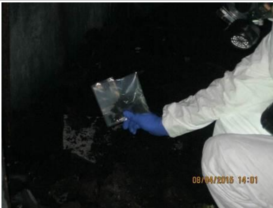
Photograph 9: Location P001-BA-009 in west wing basement. The sample was collected from a debris pile on floor. Analytical results indicate that the sample was non-detect for asbestos.
