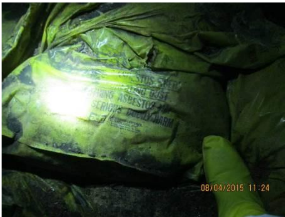
Photograph 3: Location P001-BA-003 in the west wing basement. The sample was collected from material outside of “Asbestos” labeled bags. Analytical results indicate that the sample contains 33.30% chrysotile asbestos.
