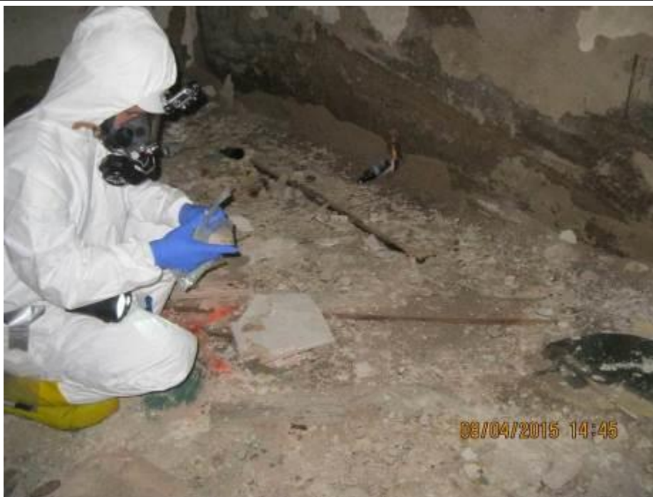
Photograph 11: Location P001-BA-011 in east wing basement. The sample was collected from floor tile. Analytical results indicate that the sample was non-detect for asbestos.
