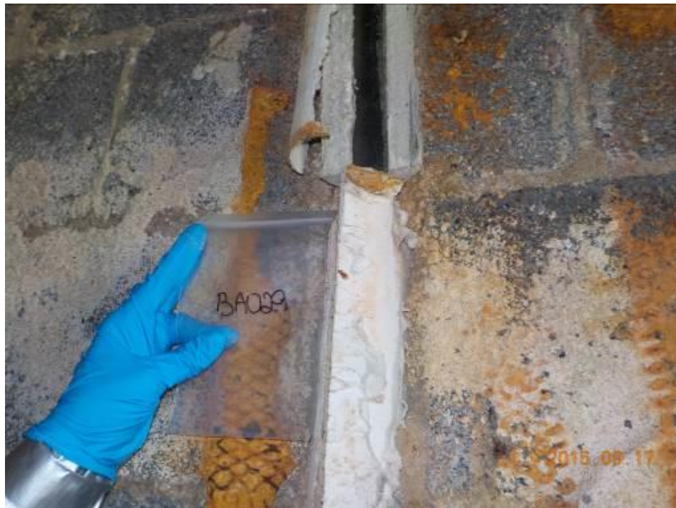
Photograph 34: Location P001-BA-029. The sample was collected from pipe wrap protruding from wall. The pipe is partially embedded in the wall. There is an adjacent pipe and pipe wrap similar to this. Several broken/open windows are located in the room. Analytical results indicate that the sample contains 30.80% chrysotile asbestos.
