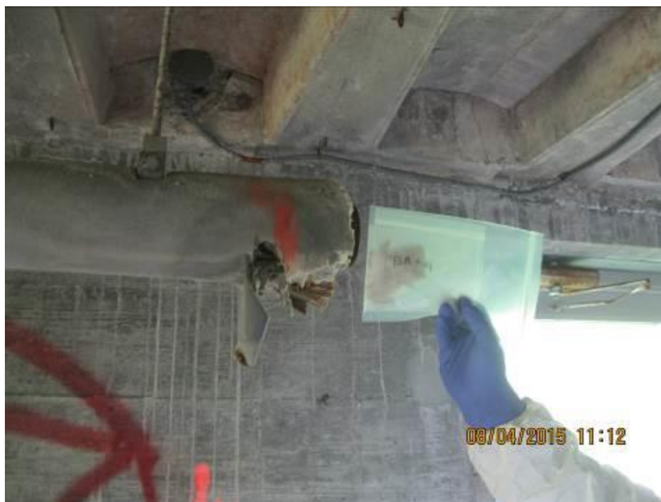
Photograph 1: Location P001-BA-001 in the west wing basement. The sample was collected from pipe insulation. Analytical results indicate that the sample contains 44.40% chrysotile asbestos.
