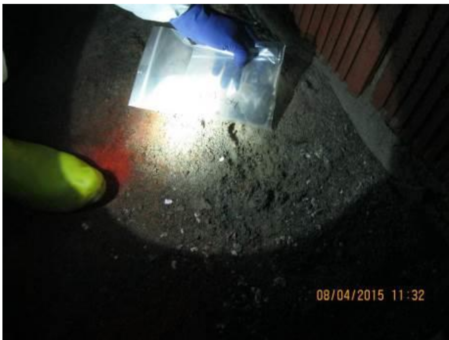
Photograph 4: Location P001-BA-004 in west wing basement. The sample was collected from a debris pile on the floor. Analytical results indicate that the sample was non-detect for asbestos.
