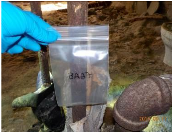
Photograph 32: Location P001-BA-027. The sample was collected from deteriorated pipe wrap at the base of a vertical pipe. Analytical results indicate that the sample contains 44.40% chrysotile asbestos.
