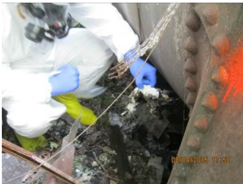
Photograph 20: Location P001-BA-020 outside of the building, approximately 15 feet to the north in a pit. The sample was collected from insulation on a suspect tank. Analytical results indicate that the sample contains 36.40% chrysotile asbestos.
