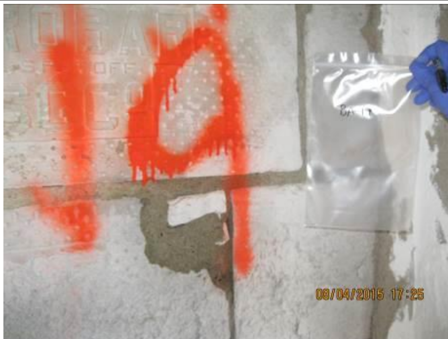
Photograph 19: Location P001-BA-019 in east wing first floor. The sample was collected from pyrobar/mortar material. Analytical results indicate that the sample was non-detect for asbestos.
