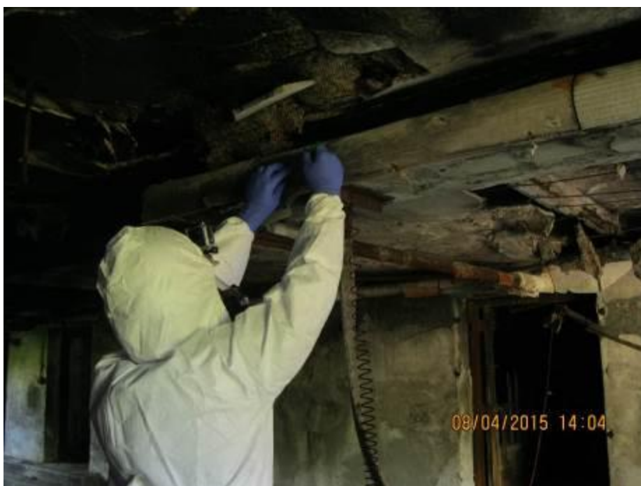
Photograph 10: Location P001-BA-010 in the west wing basement. The sample was collected from pipe insulation. Analytical results indicate that the sample contains 21.10% chrysotile asbestos.
