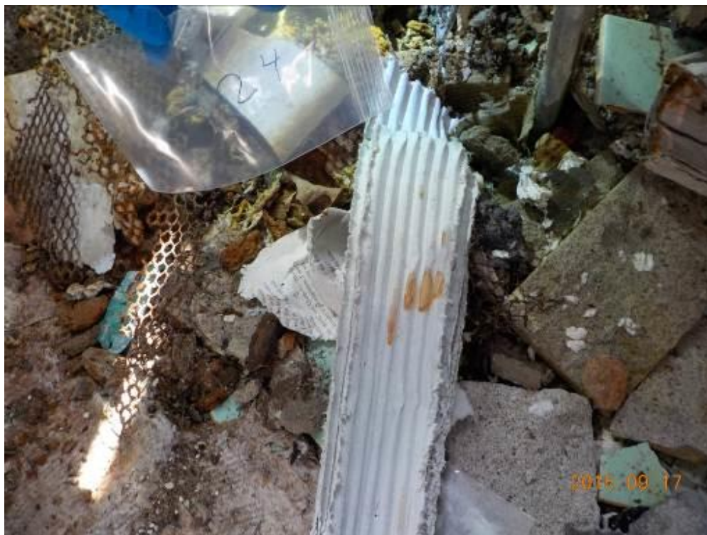
Photograph 29: Location P001-BA-024. The sample was collected from pipe wrap fallen onto floor. Analytical results indicate that the sample contains 57.10% chrysotile asbestos.
