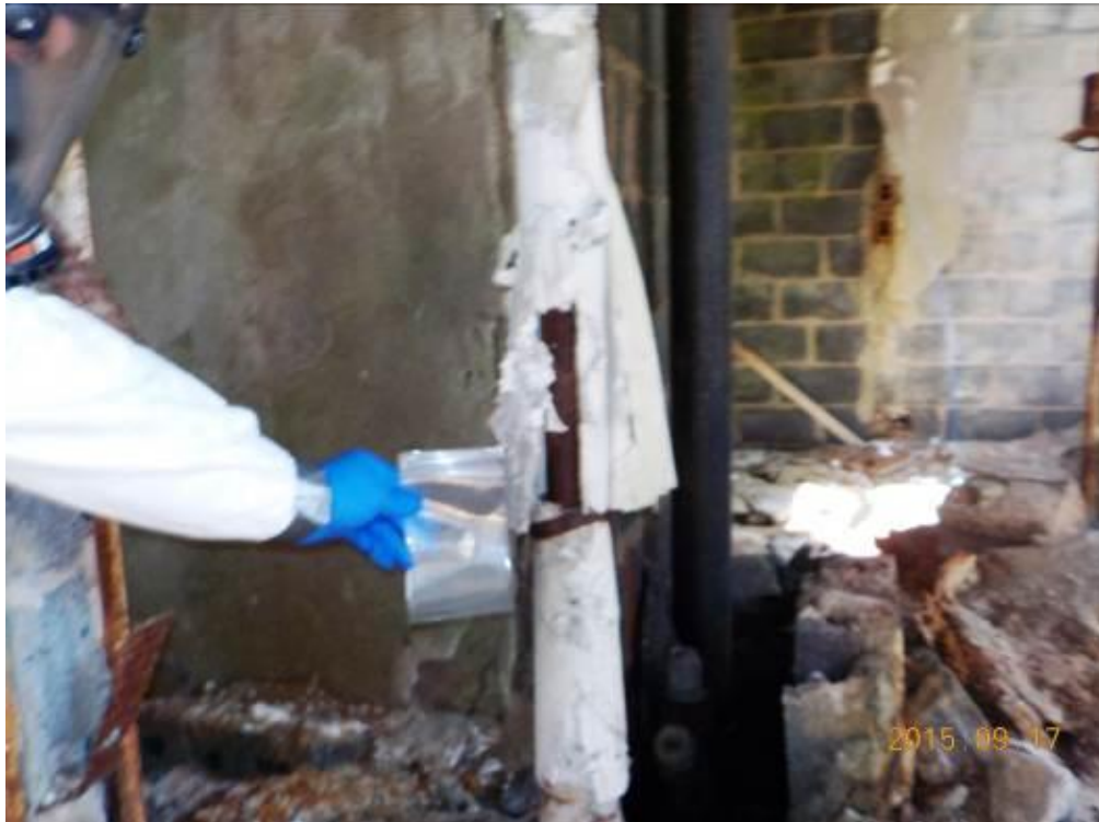
Photograph 35: Location P001-BA-030. The sample was collected from deteriorated pipe wrap on vertical pipe. Analytical results indicate that the sample contains 50.00% chrysotile asbestos.
