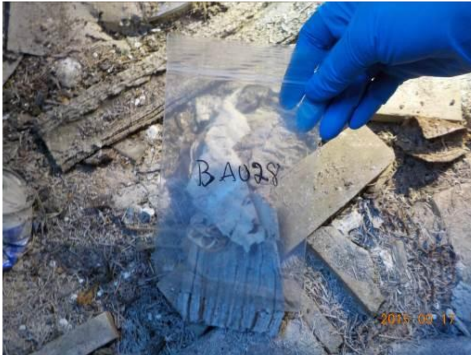
Photograph 33: Location P001-BA-028. The sample was collected from pipe wrap on floor. Analytical results indicate that the sample contains 57.10% chrysotile asbestos.
