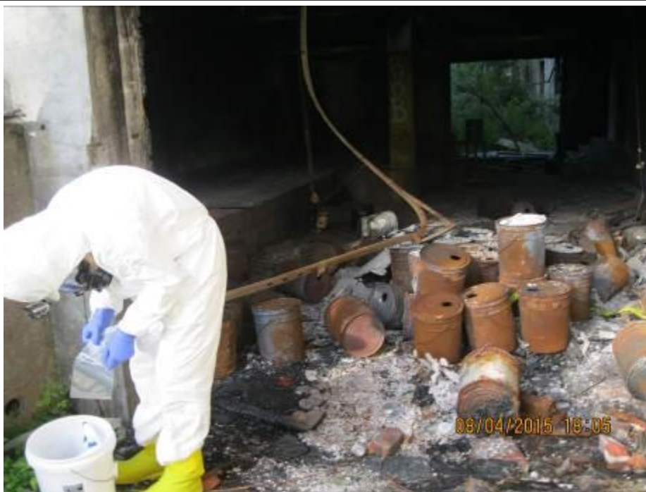
Photograph 21: Location P001-BA-021 outside the northwest entrance to the building, adjacent to sample location P001-BA010. The sample was collected from a debris pile. Analytical results indicate that the sample contains 36.40% chrysotile asbestos.
