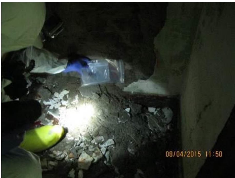
Photograph 7: Location P001-BA-007 in west wing basement. The sample was collected from a debris pile on the floor. Analytical results indicate that the sample was non-detect for asbestos.
