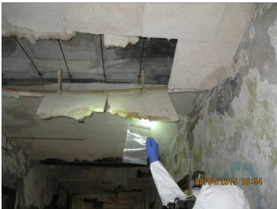
Photograph 16: Location P001-BA-016 in west wing first floor. The sample was collected from ceiling tile. Analytical results indicate that the sample was non-detect for asbestos.
