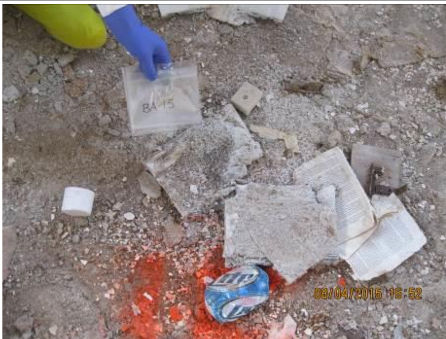
Photograph 15: Location P001-BA-015 in west wing first floor. The sample was collected from ceiling tile that had fallen to the floor. Analytical results indicate that the sample was non-detect for asbestos.
