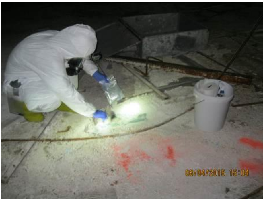
Photograph 14: Location P001-BA-014 in east wing basement. The sample was collected from a debris pile on floor. Analytical results indicate that the sample contains 5.40% chrysotile asbestos.
