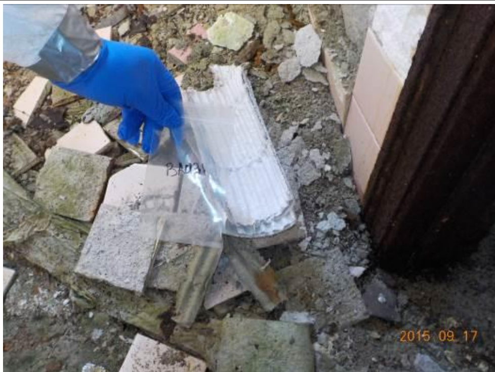
Photograph 37: Location P001-BA-031. The sample was collected from pipe wrap fallen onto floor from overhead pipe. Analytical results indicate that the sample contains 57.10% chrysotile asbestos.
