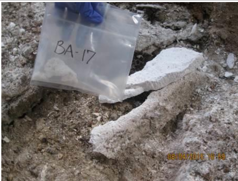
Photograph 17: Location P001-BA-017 in west wing first floor. The sample was collected from degrading ceiling tile. Analytical results indicate that the sample was non-detect for asbestos.
