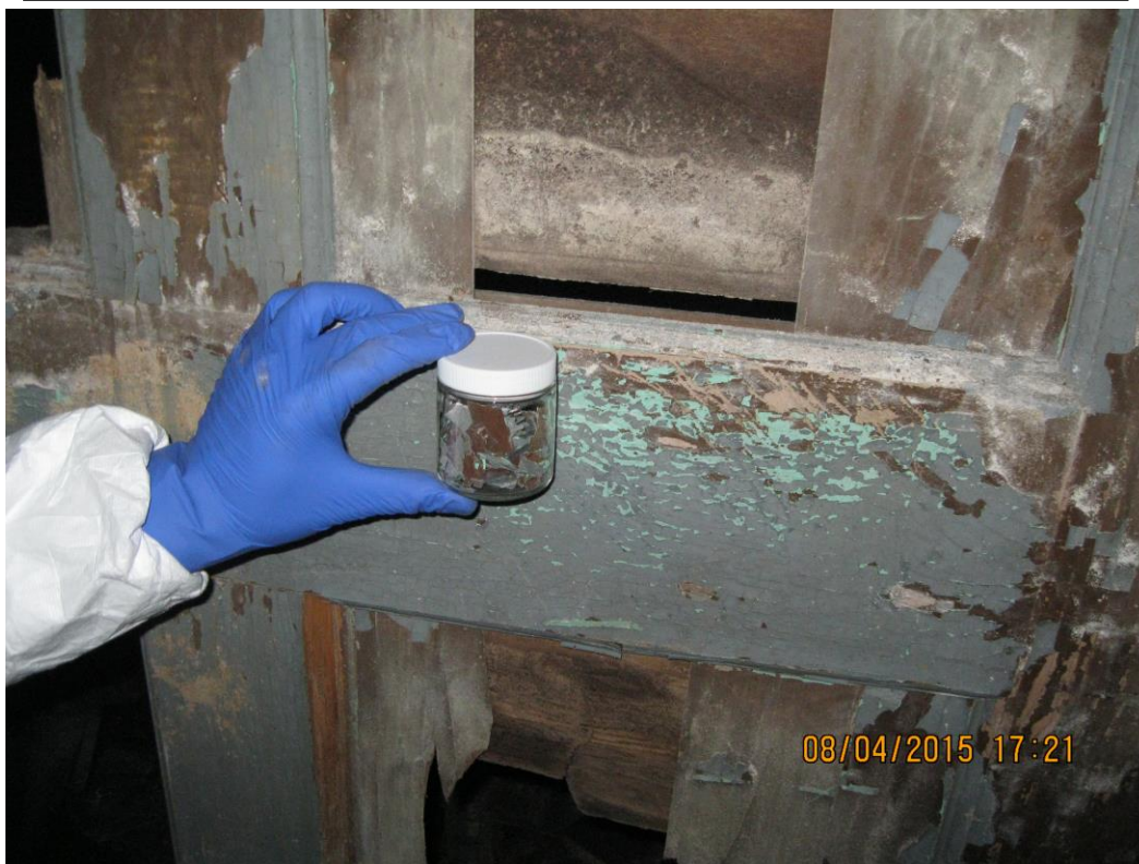
Photograph 39: Location P001-PC-001. The paint chip sample was collected in basement and analyzed for toxicity characteristic leaching procedure (TCLP) metal analysis (barium, cadmium, and lead only). The results were 127 J micrograms per liter ( \mu\text{g/L} ) for barium, 26.6 J \mu\text{g/L} for cadmium, and 41,100 \mu\text{g/L} for lead.
