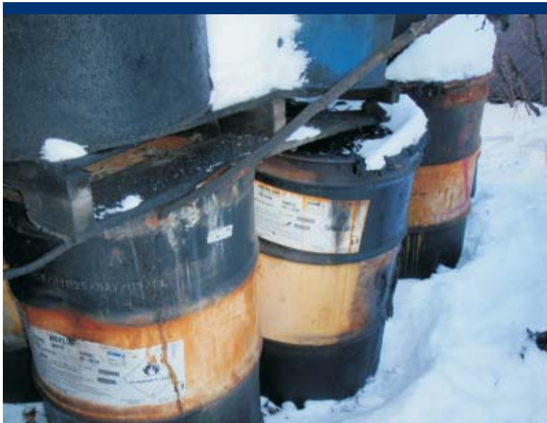
Photo 10 Drums in the "GRW" area that displayed apparent spillage or leakage of a material inconsistent with the type of product indicated by drum labeling information.
