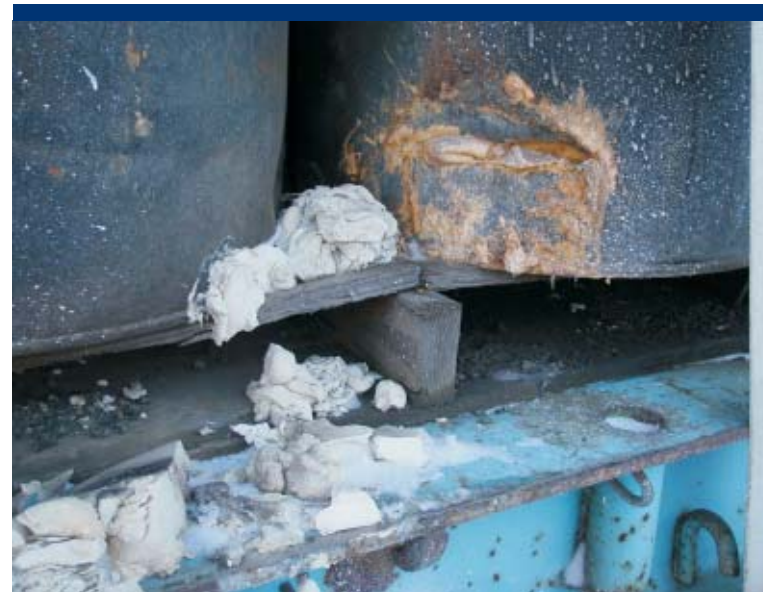
Photo 6 Examples of damaged drums and poor-condition pallets found on the "SE" flatbed trailer.
