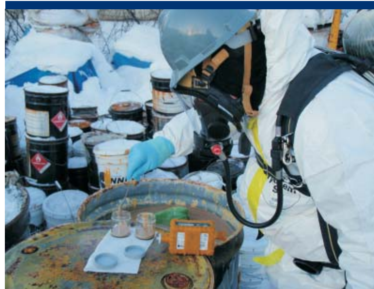
Photo 22 START collecting a field screening sample from container number 9-SE.
