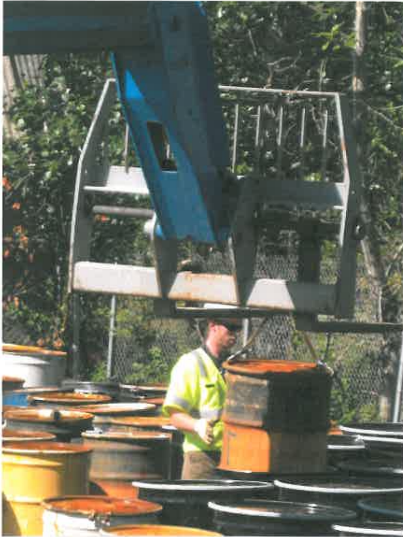
Over Packing of Drums
