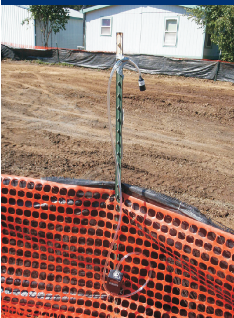
Photo 11 Example of air sampling pump and cassette.
