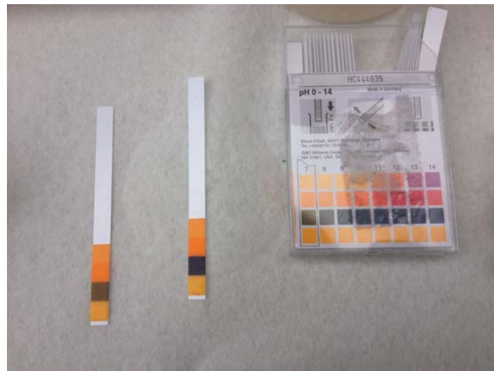
Photo No. IMG_3100; Taken on 10/01/15 at 15:37 hours by START-JW. Facing Down. pH paper while field preserving the samples. One piece of paper was from unpreserved sample water (left) the other is after preservation (right) to test a new formulation of preservation from the lab. This was not used as a sample during this sampling event.
