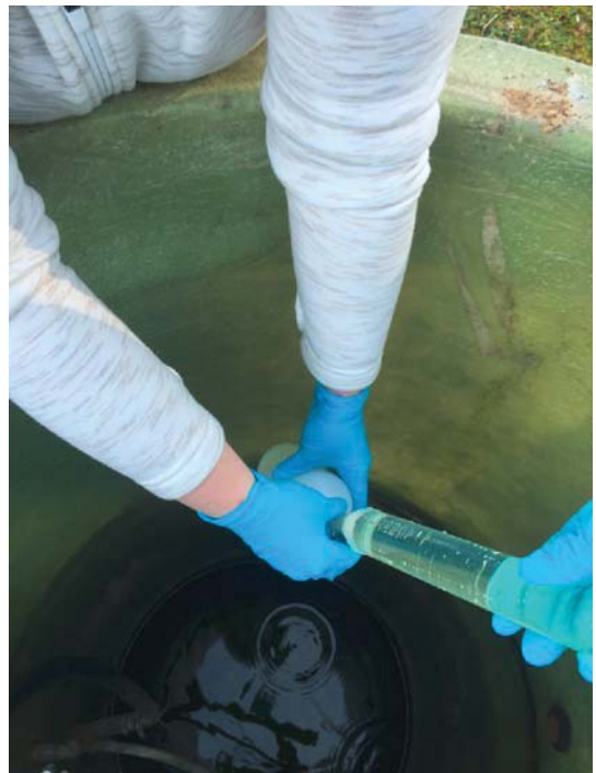
Photo No. IMG_3140; Taken on 12/09/15 at 14:02 hours by START-ET. Facing Down. TechLaw Scientists using the bailer to collect WG-SP-0003/dup WG-SP-0004.
