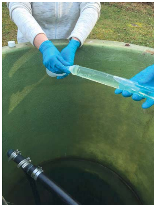
Photo No. IMG_3141; Taken on 12/09/15 at 14:03 hours by START-ET. Facing Down. TechLaw Scientists using the bailer to collect WG-SP-0003/dup WG-SP-0004.
