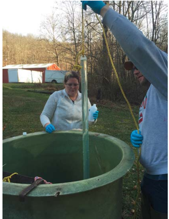
Photo No. IMG_3138; Taken on 12/09/15 at 14:02 hours by START-ET. Facing South. TechLaw scientists using a bailer to collect a sample from the primary sump location.
