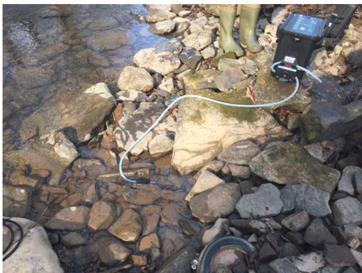
Photo No. IMG_3131; Taken on 12/09/15 at 13:08 hours by START-JW. Facing Down. The Set up used by TechLaw to collect sample WG-SW-0020
