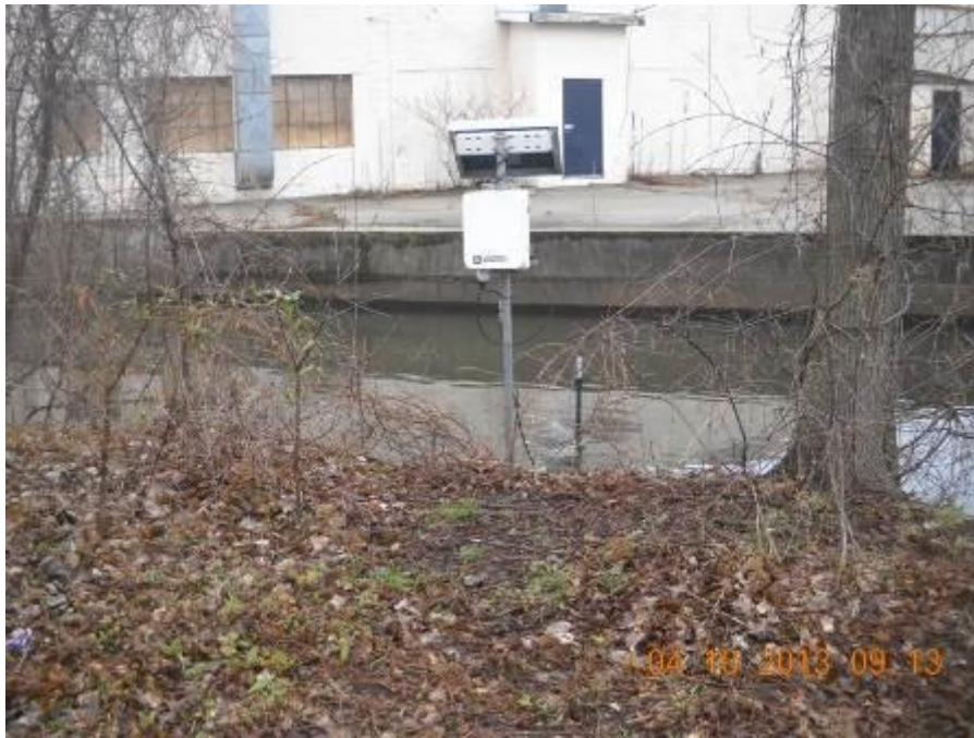
Site: Portage Creek Area Site – SA5-A Photograph No.: 19 Direction: East Subject: Turbidity monitor located upstream
