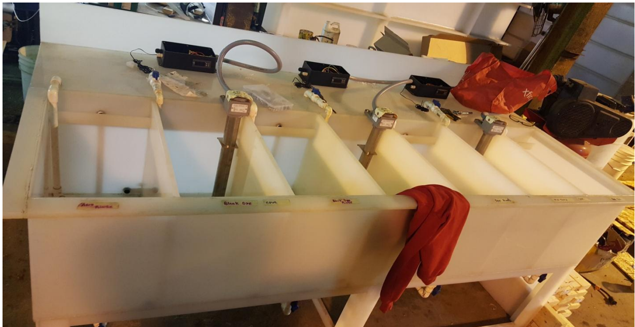
Photo 10 – Showing custom built electroplating tanks
