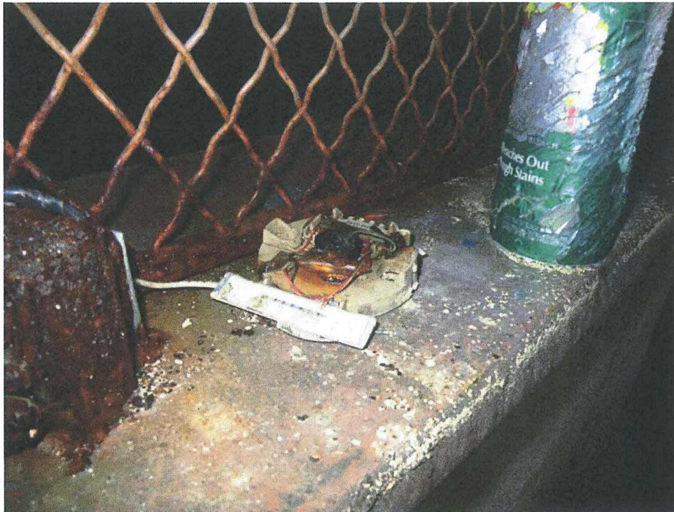
Photo11: Damaged thermostat containing mercury
