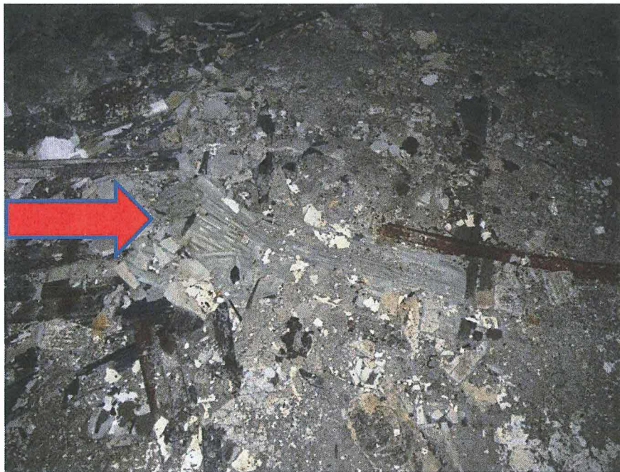
Photo 6: Comingled friable asbestos (pipe wrap) and lead/PCB paint pulverized on floor
