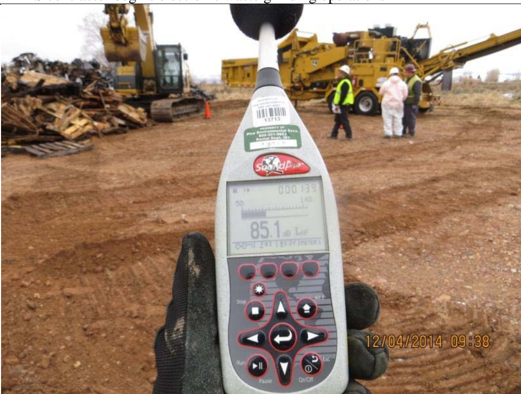
Photo Number: IMG_C02.JPG Date: 12/4/14 Direction: Northwest Photographer: Bryniarski Subject: START contractor collects noise level readings during grinding operations
