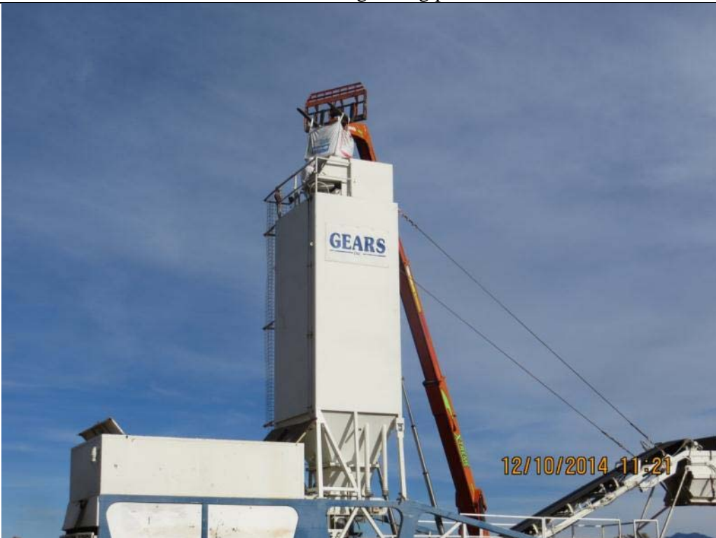
Photo Number: IMG_G03.JPG Date: 12/10/14 Direction: Northeast Photographer: Bryniarski Subject: ERRS contractor loads cement into silo of pug mill prior to second waste treatment process
