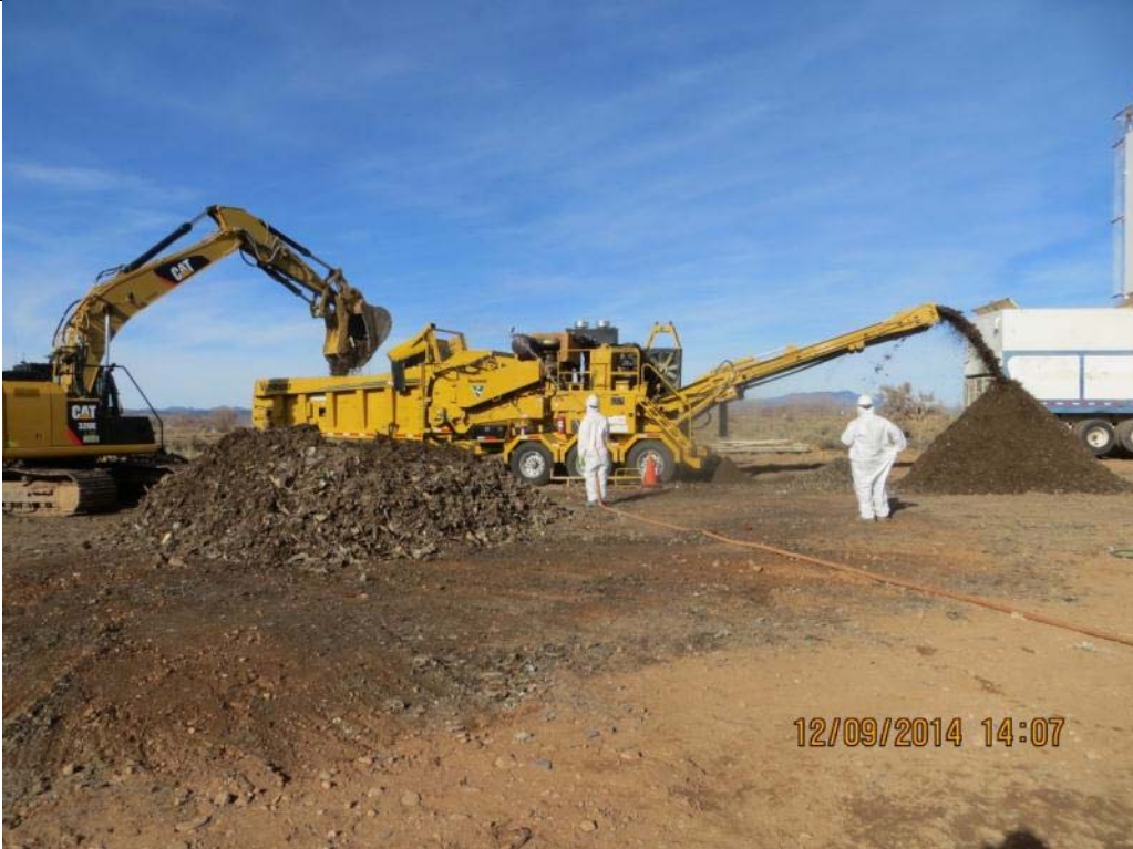
Photo Number: IMG_F09.JPG Date: 12/9/14 Direction: North Photographer: Bryniarski Subject: ERRS contractor loads waste for second grinding process
