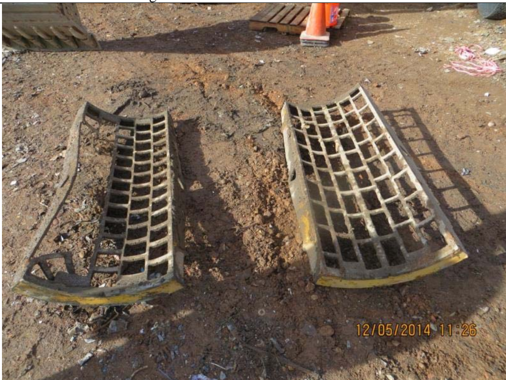
Photo Number: IMG_D03.JPG Date: 12/5/14 Direction: Overhead Photographer: Bryniarski Subject: Damaged grinder cutting screen (3-4 inch size)
