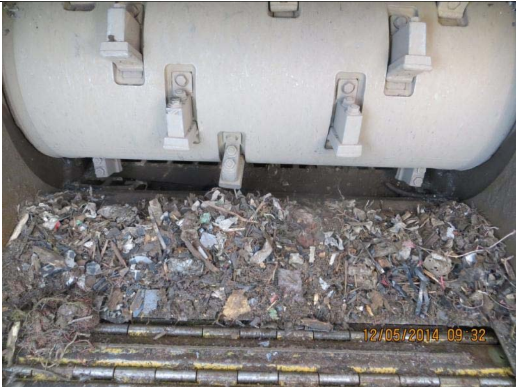
Photo Number: IMG_D02.JPG Date: 12/5/14 Direction: Overhead Photographer: Bryniarski Subject: Electronic waste inside grinder feed chamber
