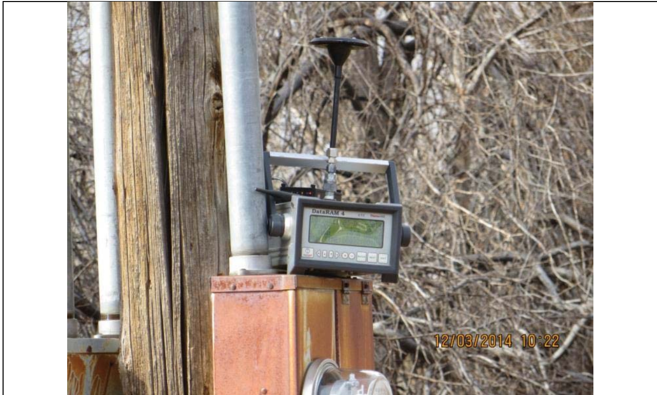
Photo Number: IMG_B03.JPG Date: 12/3/14 Direction: West Photographer: Bryniarski Subject: START contractor collects air monitoring data with Data Ram and VIPER Linc
