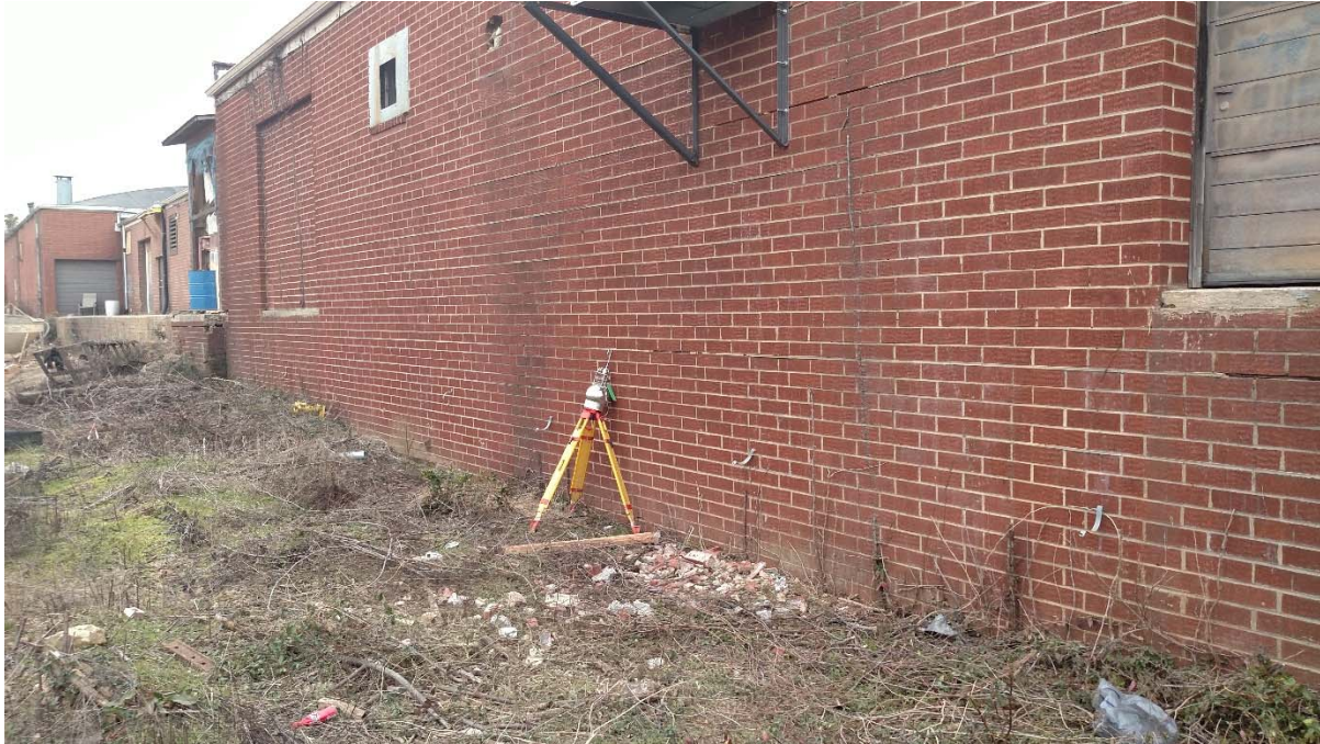
Photo #7: Summa canister deployed to collect an ambient air sample on the south side of the Leather Trimmings building.
