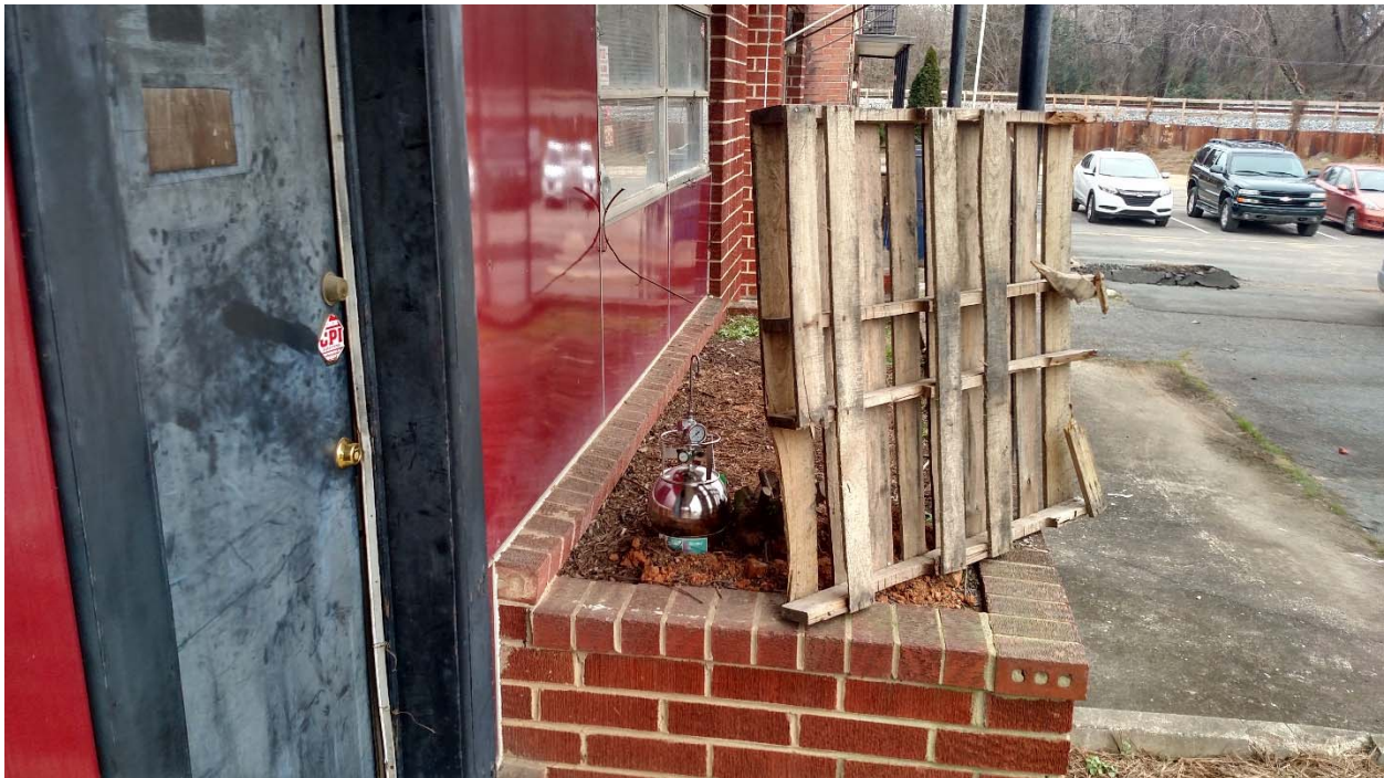
Photo #6: Summa canister deployed for collection of an ambient air sample on the north side of the Leather Trimmings building.
