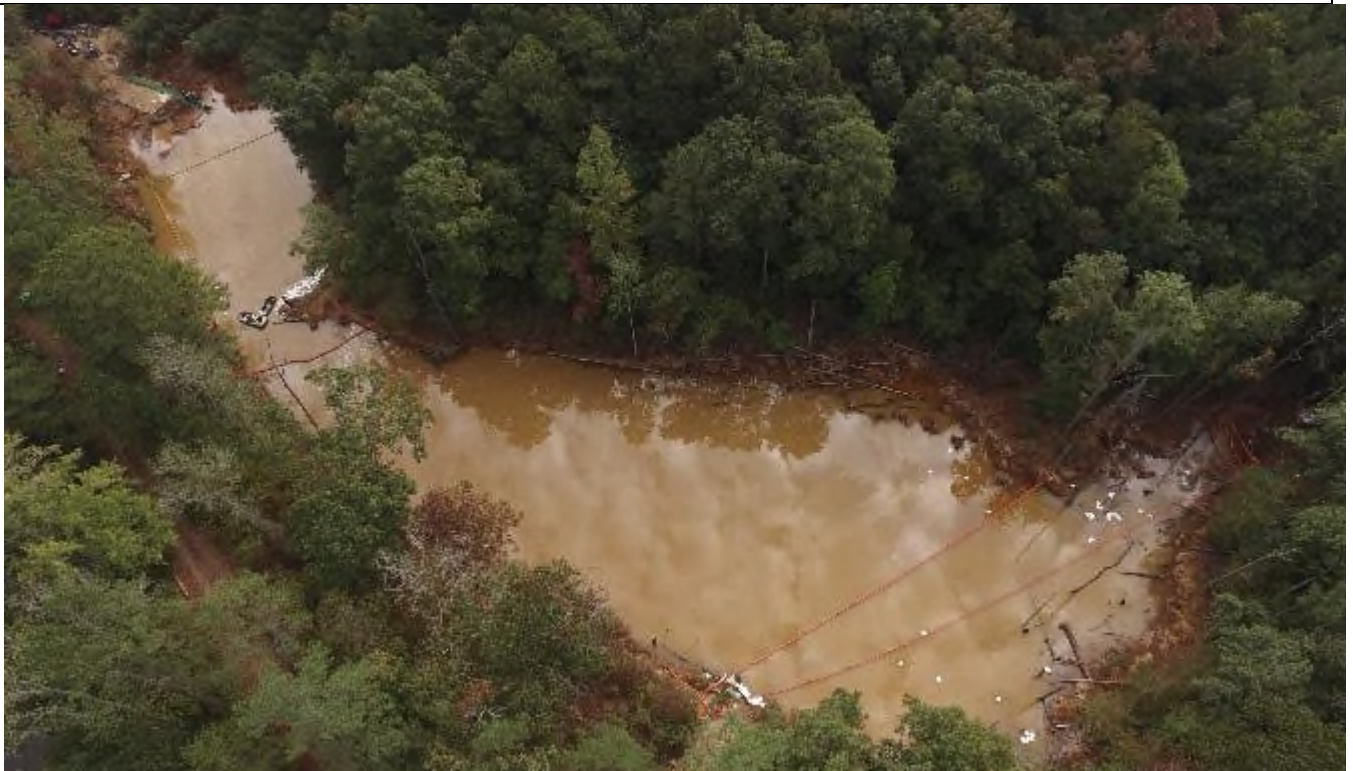
Latest aerial showing reduction in fuel coverage and installation of protective shore boom.
